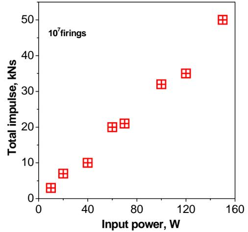
**Figure 1. Total impulse – Input power dependence (referred to 10<sup>7</sup> firings, room temperature). RIAME developed APPTs.**
