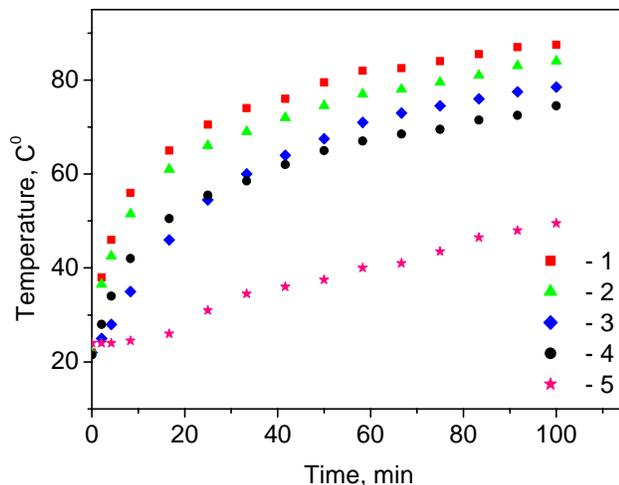
**Figure 6. Temperature of APPT elements vs duration of work at 2 Hz frequency. 1 -cathode, 2 -anode, 3- -propellant, 4- lead terminal of the capacitor, 5- lateral surface of the capacitor**
