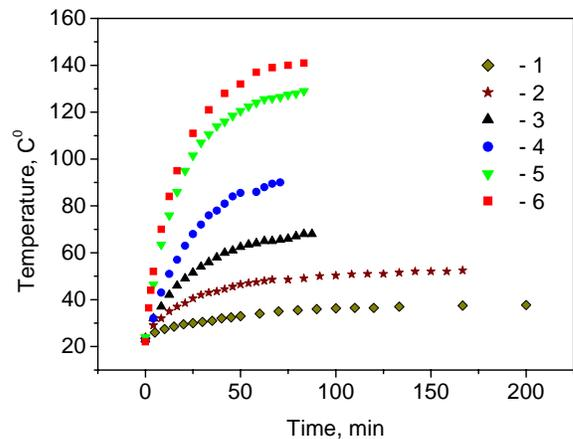
Figure 4. Propellant bar temperatures in dependence on duration of APPT work at various frequencies. 1 -  $f=0.2$  Hz,  $m=0.07$  mg; 2 -  $f=0.5$  Hz,  $m=0.074$  mg; 3-  $f=1$  Hz,  $m=0.078$  mg; 4-  $f=2$  Hz,  $m=0.084$  mg; 5 -  $f=3$  Hz,  $m=0.087$  mg; 6 -  $f=3$  Hz,  $m=0.092$  mg.
