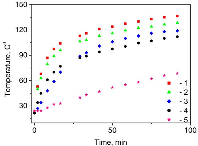
**Figure 5 - Temperature of APPT elements vs duration of work at 4 Hz frequency. 1 -cathode, 2 -anode, 3- -propellant, 4- lead terminal of the capacitor, 5- lateral surface of the capacitor**
