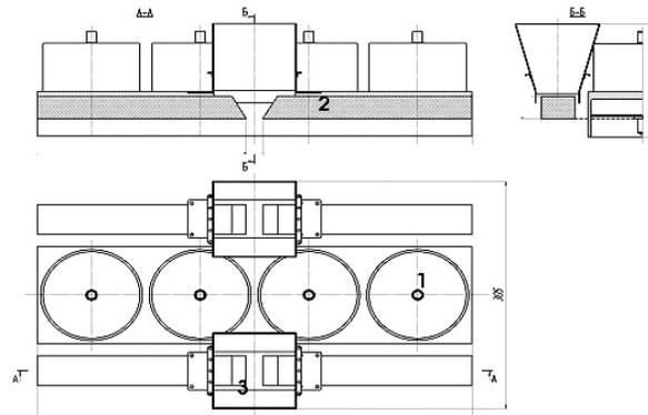
Figure 2. APPT-95 assembly, 1 – capacitors, 2 – propellant bar, 3 – acceleration channel.
