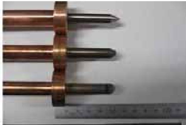
**Figure 7. Photos of eroded cathodes.**
