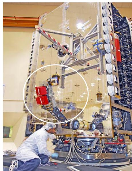
Figure 15. DSM range of motion testing using spacecraft offloader.
