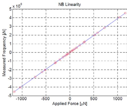
**Figure 7: Relationship between applied force and measured frequency variations extended up to  $\approx \pm 1$  mN range**
