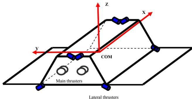
Figure 1: Arrangement of two main thrusters and eight lateral thrusters on the satellite for the NGGM
