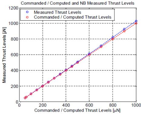
**Figure 11: Nanobalance measured whole thrust characteristic vs. commanded / computed thrust**
