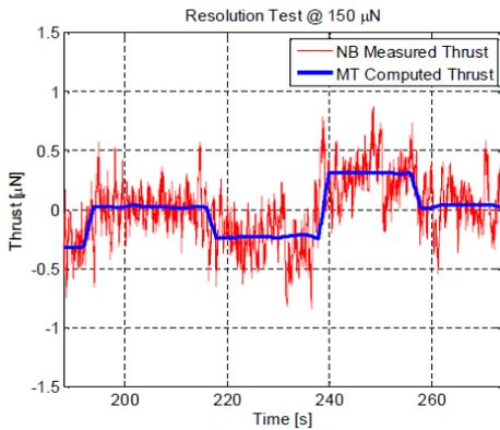
**Figure 12: Thrust resolution**
