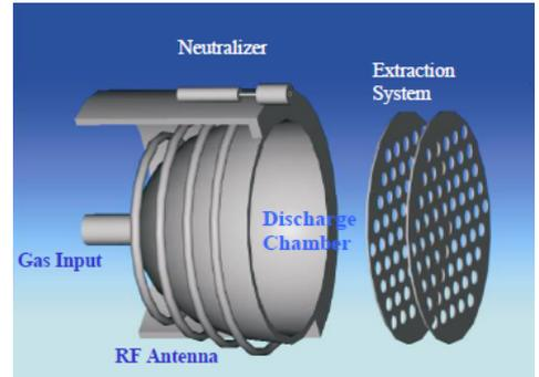
Figure 4: Functional principle of RIT
