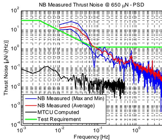
**Figure 13: Thrust noise**
