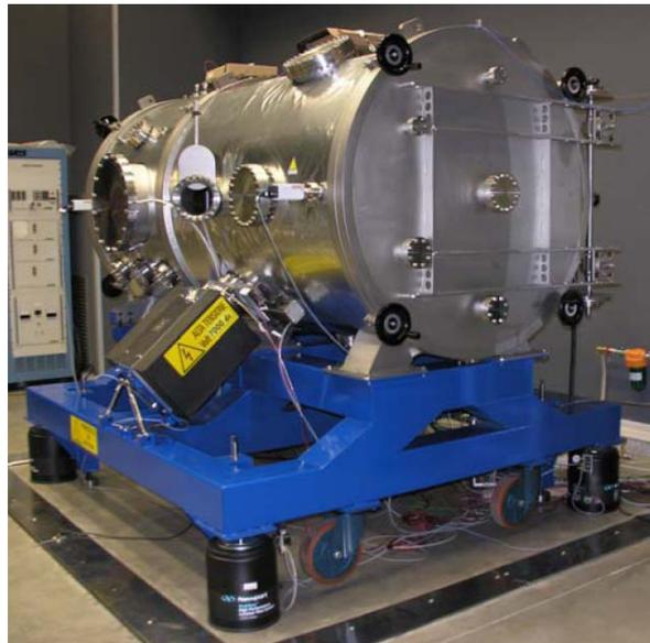
**Figure 8: Vacuum chamber hosting the Nanobalance thrust stand**
