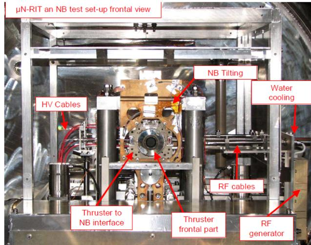
**Figure 9: Test set up**
