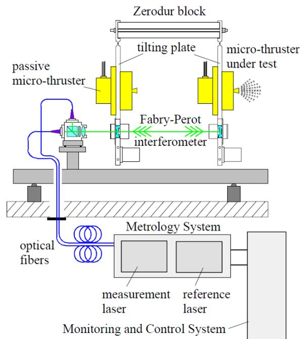
Figure 6: Block diagram of the Nanobalance
