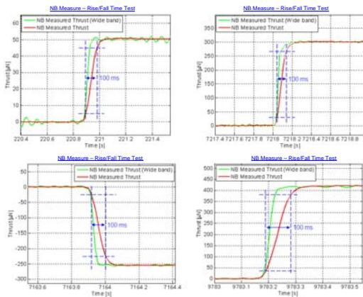
**Figure 14: Thrust rise/fall time**
