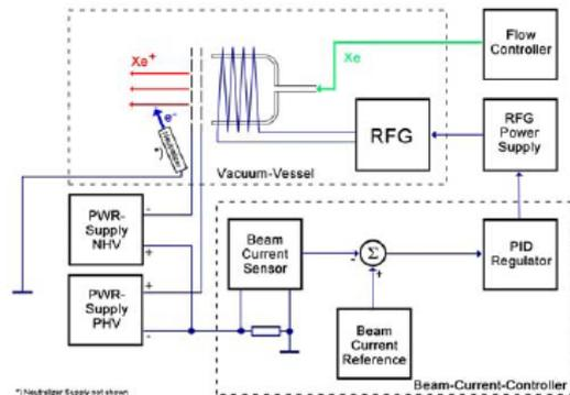
Figure 5: Block diagram of beam current control loop
