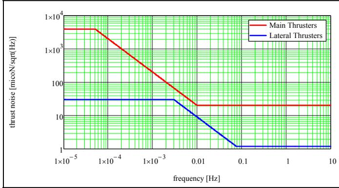
Figure 3: Preliminary requirements on the noise ( $\mu\text{N}/\sqrt{\text{Hz}}$ ) of the main and lateral thrusters
