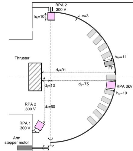
**Fig. 4. Positions of the diagnostics during plume measurements.**
