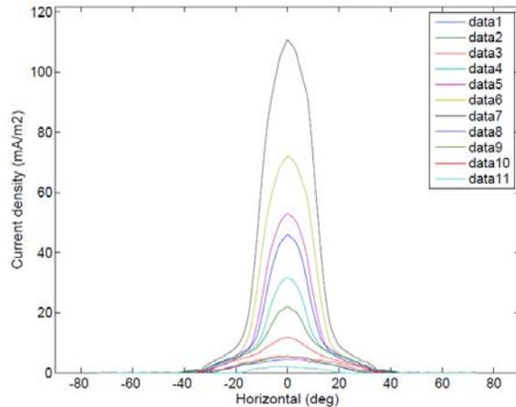
**Fig. 8. Ion beam profile measured for a thrust level of  $500 \mu N$ , neutralizer off and thruster housing grounded**
