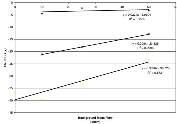
**Fig. 13. Influence of the backpressure on the CRP for three different thrust levels: 100  $\mu\text{N}$  (blue), 250  $\mu\text{N}$  (red), 500  $\mu\text{N}$  (yellow).**
