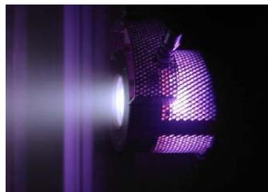
**Fig. 1. Miniaturized RIT-4 ion engine from Gießen University.**
