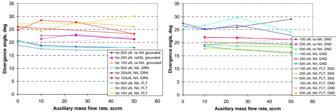
**Fig. 9. Influence of the auxiliary mass flow rate (residual neutral backpressure) on the thruster divergence for 100  $\mu\text{N}$ , 250  $\mu\text{N}$ , and 500  $\mu\text{N}$ . The thruster housing was grounded (left) or electrically isolated (right).**
