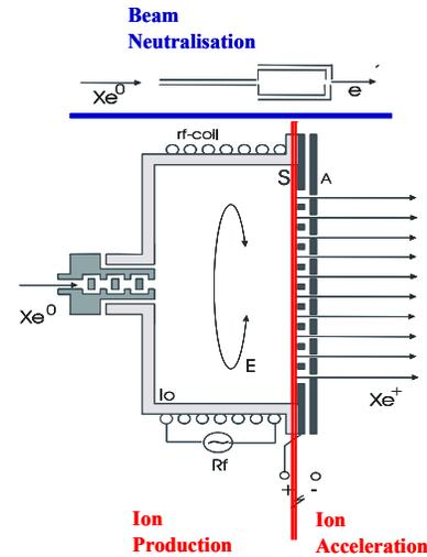
Fig. 2. RF-ion thruster function principle.
