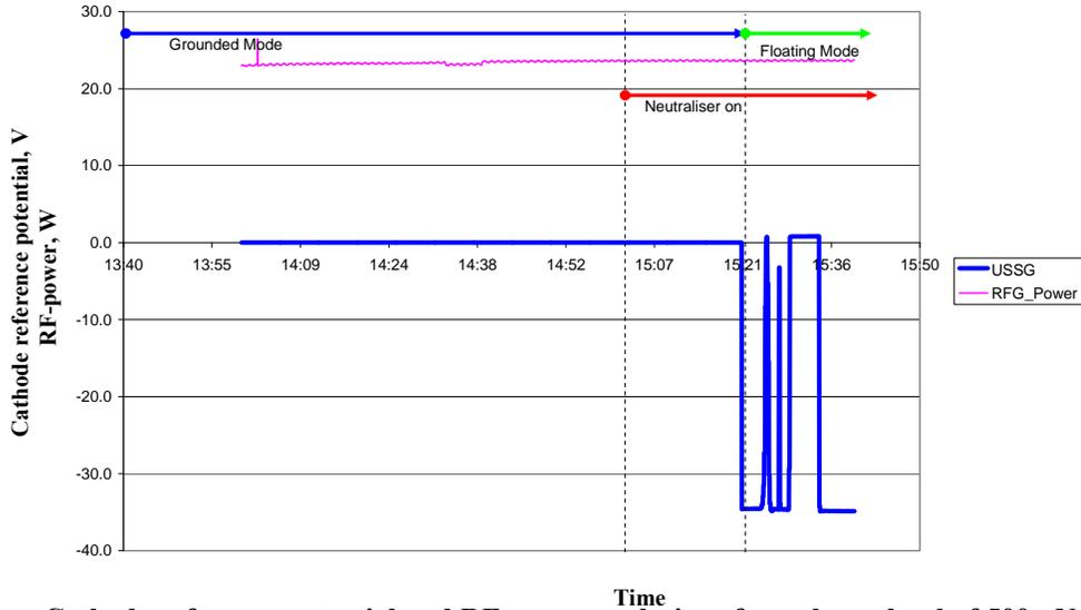
**Fig. 11. Cathode reference potential and RF-power evolutions for a thrust level of 500  $\mu\text{N}$  in function of the electrical configuration of the neutralizer. The thruster housing was grounded.**
