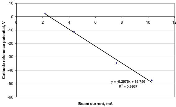
**Fig. 12. Influence of the beam current on the Cathode reference potential.**
