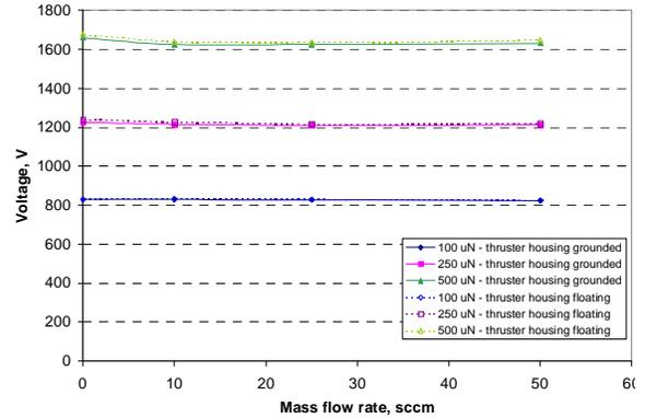
**Fig. 6. Voltage of the main peak in the ion energy distribution (3 kV RPA measurements) as a function of the background pressure (mass flow rates) and for different electrical configurations of the thruster and for the three operating regimes (blue for 100  $\mu\text{N}$ , magenta for 250  $\mu\text{N}$ , green for 500  $\mu\text{N}$ ) with neutralizer off.**
