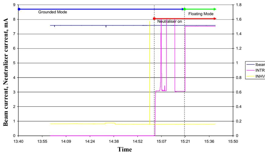
**Fig. 10. Ion beam (blue) and neutralizer (magenta) currents evolutions in function of the electrical configuration of the neutralizer, for a thrust level of 500  $\mu\text{N}$ . The thruster housing was grounded.**
