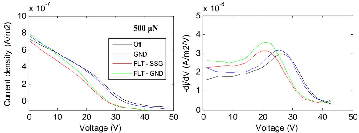
**Fig. 7. Current densities ( $A/m^2$ , left) and backflow ion distribution function ( $A/m^2/V$ , right) measured by probe 2 at  $500 \mu N$  and neutralizer conditions: off (black), on and grounded (blue), on and floating (red) and with the thruster housing floating (green).**
