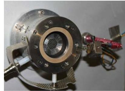
Fig. 3. RIT-4 and filament neutralizer used during the test.
