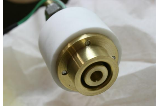
Figure 11. Coaxial SMBI and pre-ionization electrode
