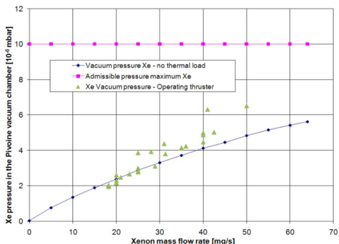
Figure 5. Pumping capabilities of the Pivoine vacuum chamber
