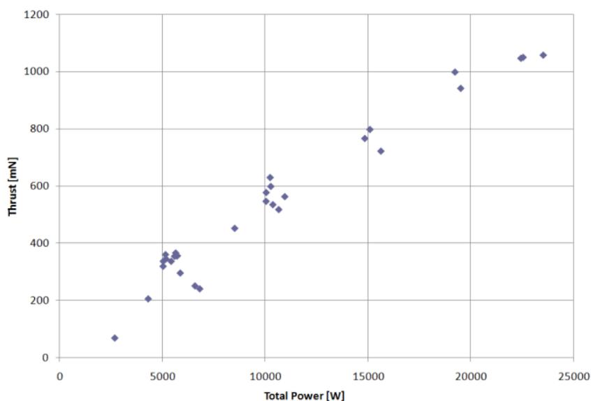
**Figure 7. Thrust versus Total Power for various discharge voltages**
