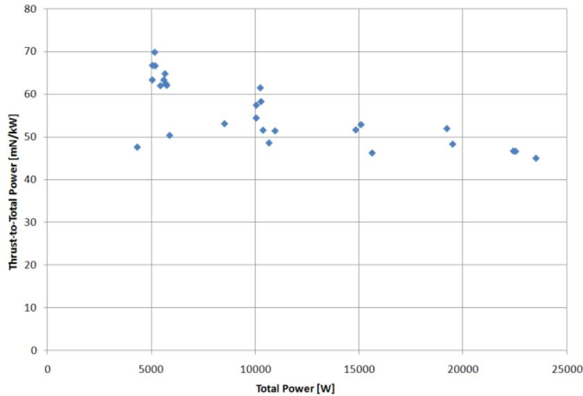
**Figure 10. Thrust-to-Total Power versus Total Power for various discharge voltages**
