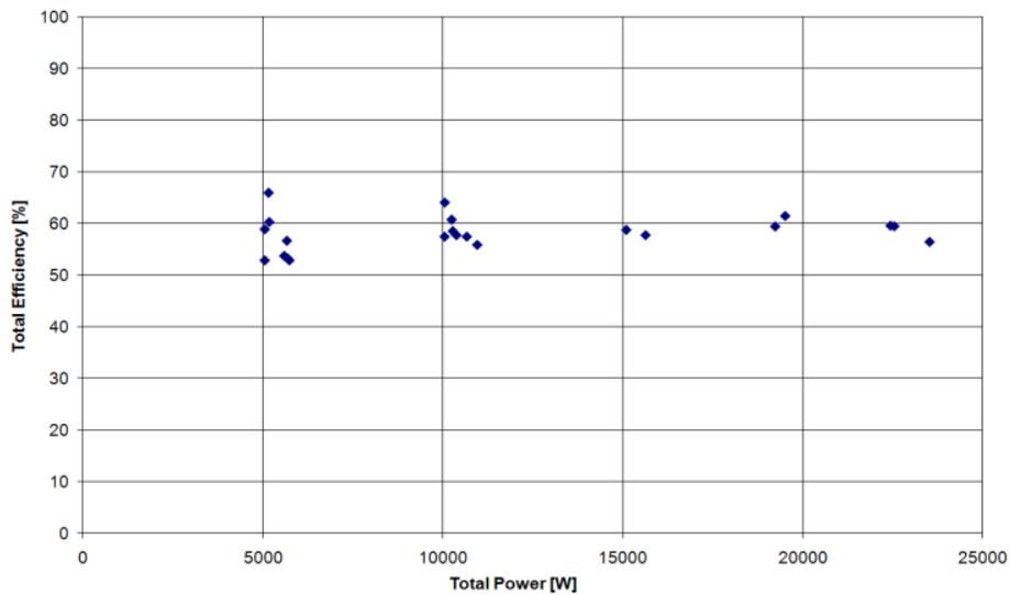
**Figure 9. Total Efficiency versus Total Power for various discharge voltages**
