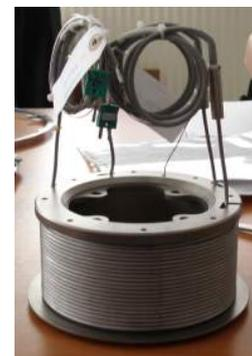
Figure 2. Internal annular coil
