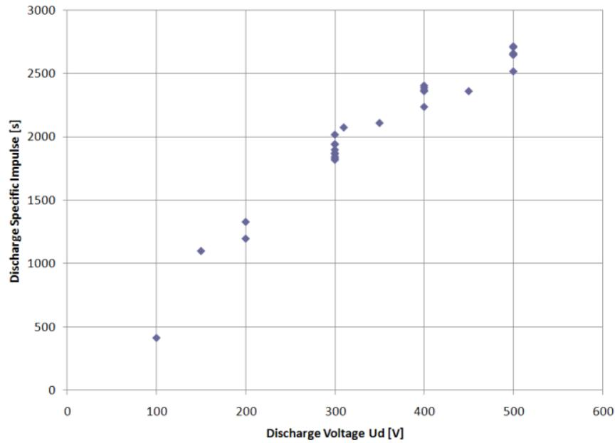
**Figure 8. Discharge specific impulse versus discharge voltage Ud**
