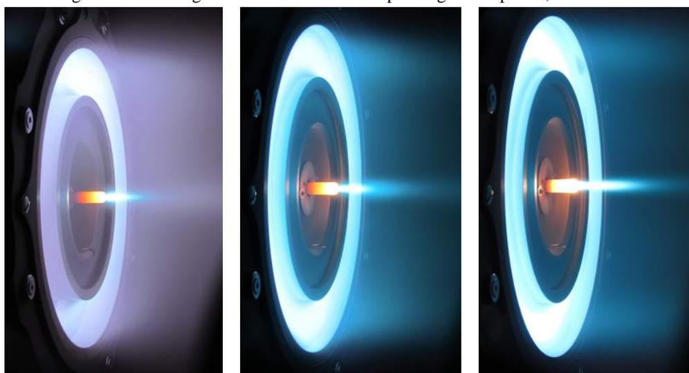
Figure 6. PPS-20k ML at low power, 15 kW and 23.5 kW
