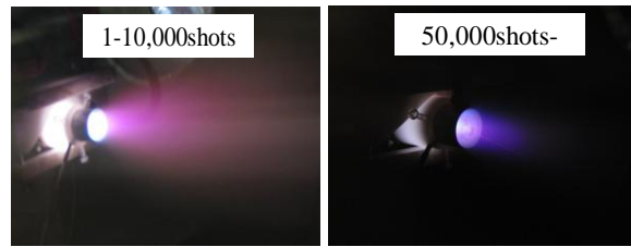
Figure 8. Feature of plasma plume. a) 1-10,000 shots, b) 50,000shots.
