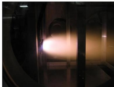
**Figure 11. Photos of plasma plume with mixture of HAN and N<sub>2</sub>.**
