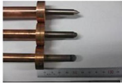
**Figure 9. Photos of eroded cathodes.**
