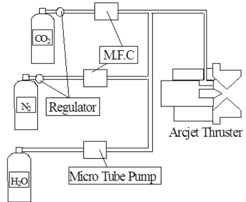
**Figure 6. Propellant supply system.**
