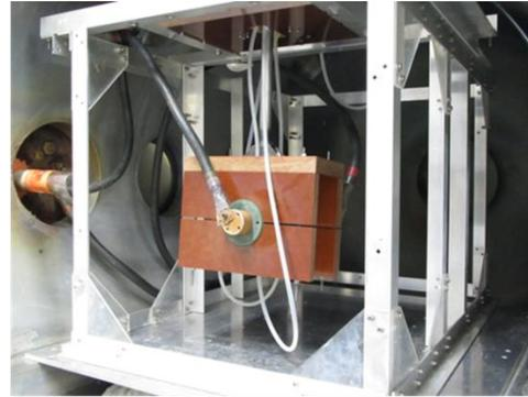
**Figure 7. Thrust measurement system.**
