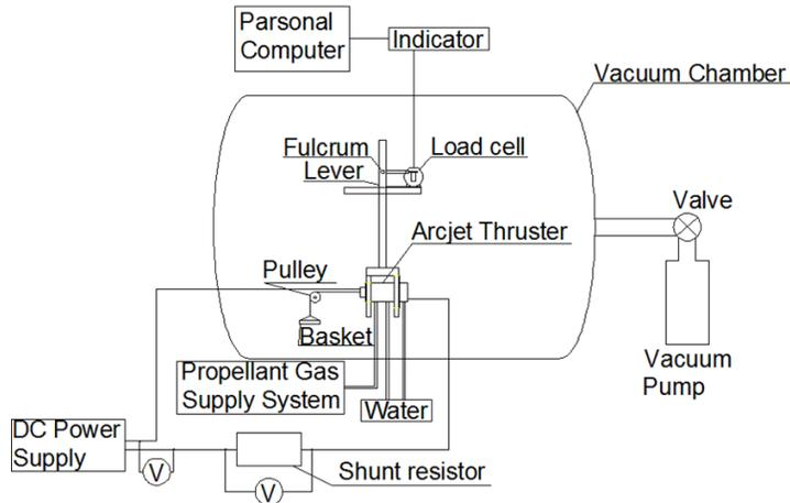
**Figure 5. Experimental system for arcjet thruster.**
