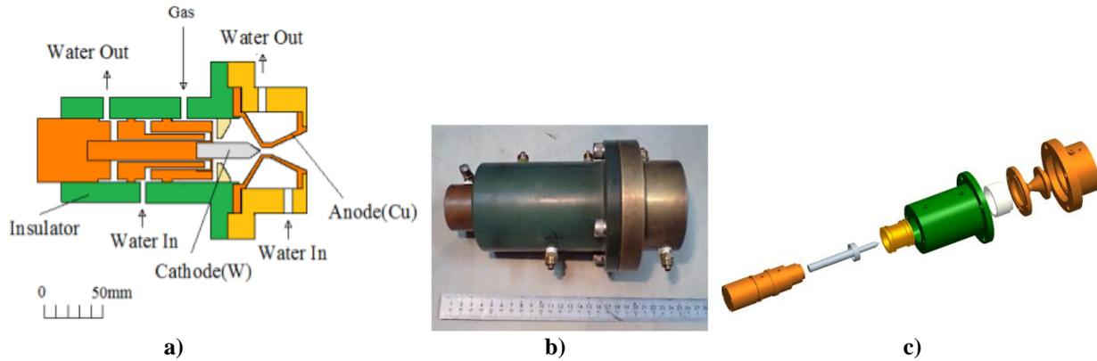
**Figure 1. Configuration of water-cooled direct-current arcjet.**
