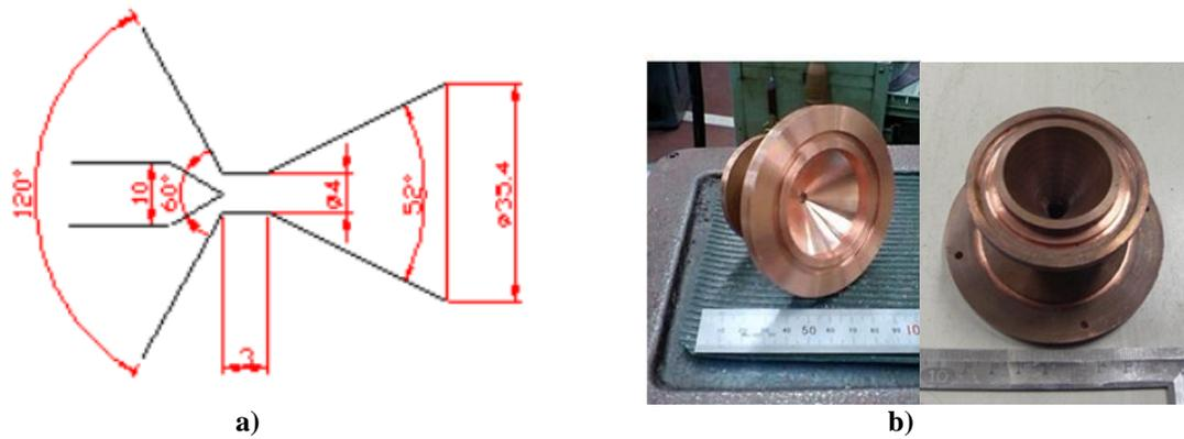
**Figure 2. Electrode configuration and anode part.**
