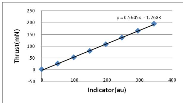
**Figure 8. Thrust calibration curve.**
