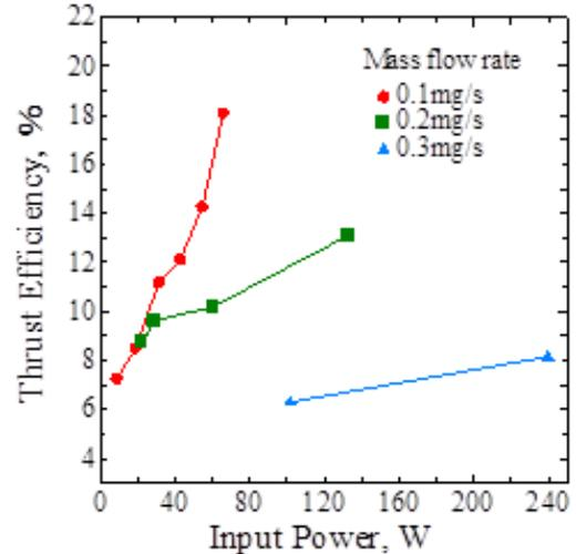
Figure 10. Thrust efficiency vs input power.
