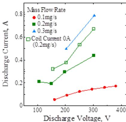
Figure 6. Discharge current vs discharge voltage.
