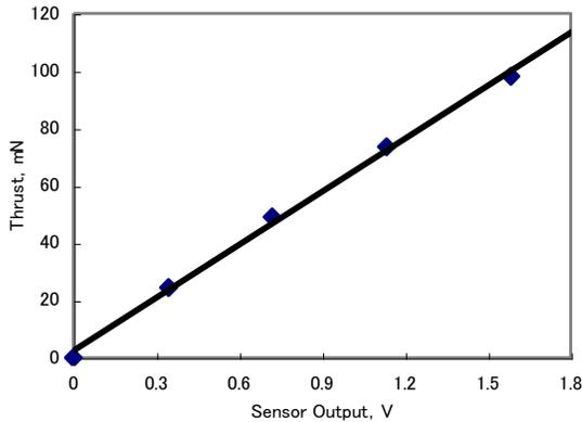
Figure 4. Typical thrust calibration line.
