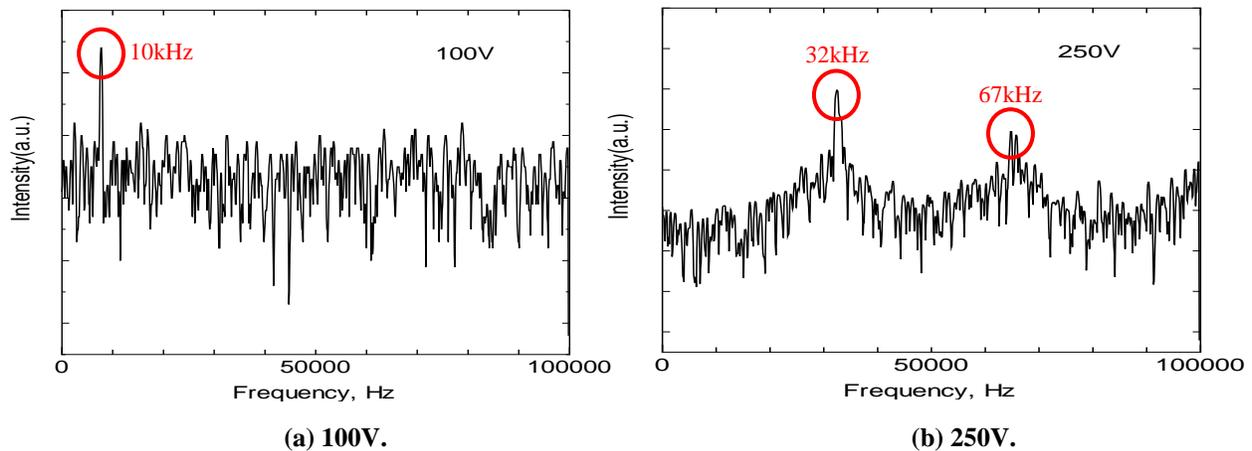
Figure 12. FFT analysis of discharge current oscillation.
