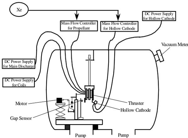
Figure 3. Experimental system for Hall Thruster.
