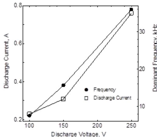
Figure 13. Discharge voltage dependence of discharge oscillation.
