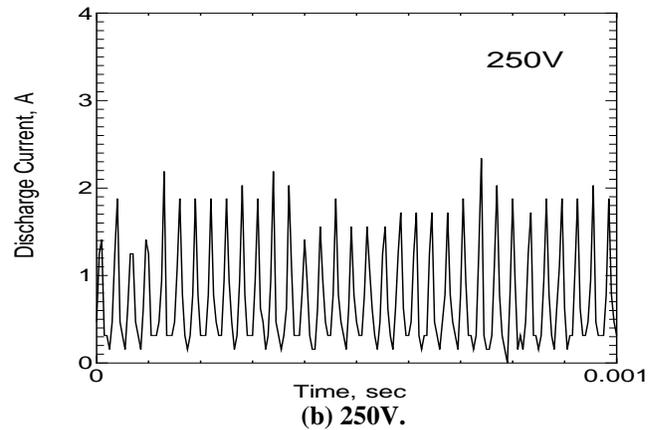
Figure 11. Oscillations of discharge current.
