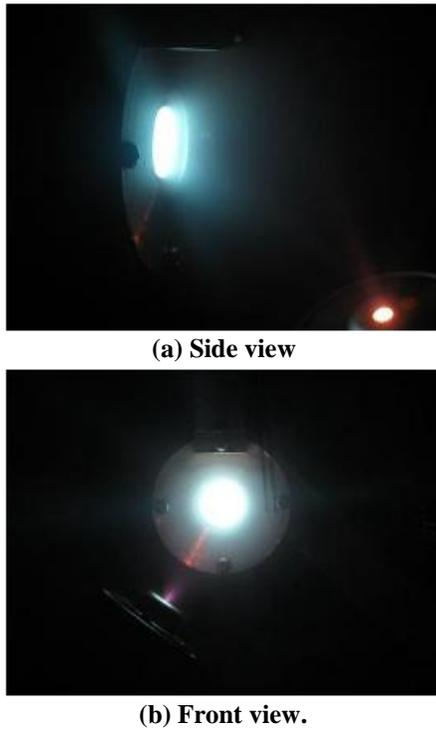
Figure 5. Typical photo of plasma plume for TCHT-4.
