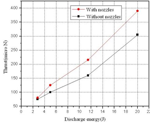
**Figure 6. Profile of the thrust in different energy level**
