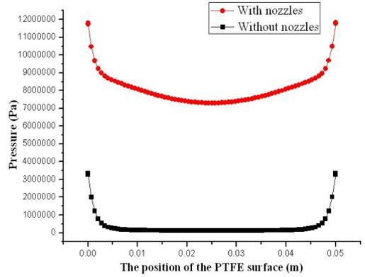
Figure 9. The comparison of pressure on the surface of PTFE
