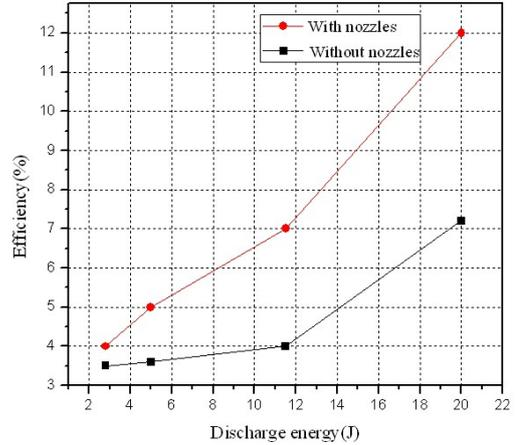
Figure 10. The profile of PPT efficiency in different energy level
