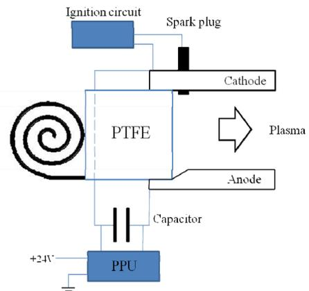
Figure 1. Basic schematic of PPT
