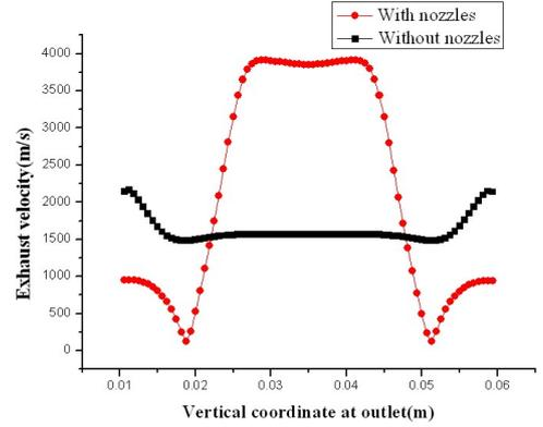
Figure 8. The comparison of the velocity on outlet
