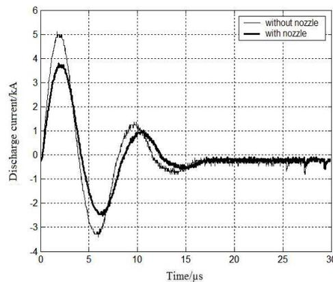
**Figure 5. The variation of discharge current with and without nozzle (5J)**
