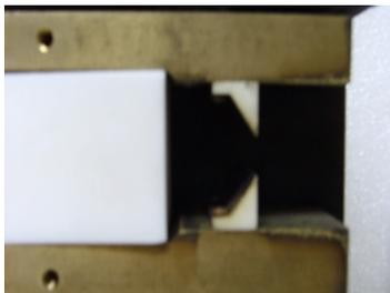
Figure 3. New electrodes with ceramic nozzles
