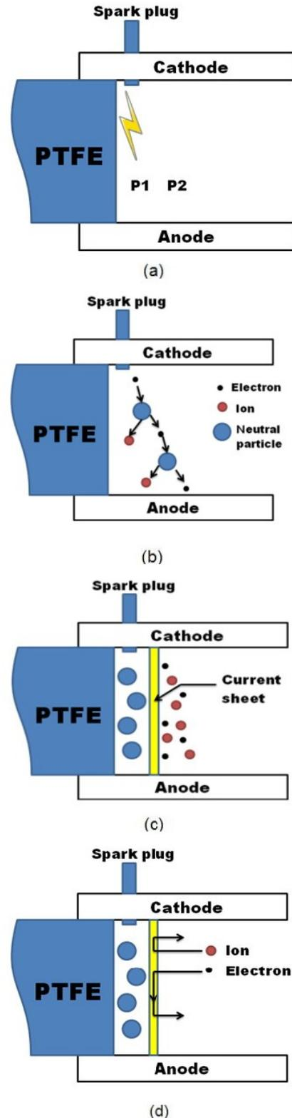
Figure 2. Acceleration processes of charged particles
