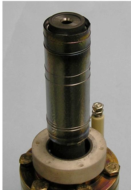
Figure 6. The 1.5-cm dia. LaB<sub>6</sub> hollow cathode with heater and heat shield installed, but without the keeper installed.
