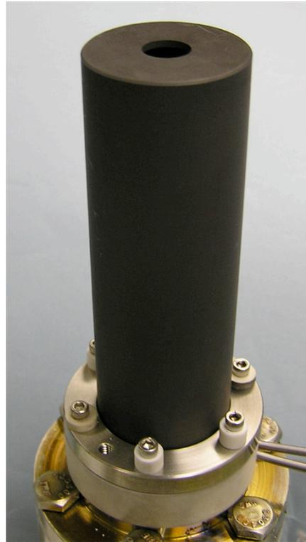
Figure 7. The 2-cm OD tube  $\text{LaB}_6$  hollow cathode with the keeper mounted.
