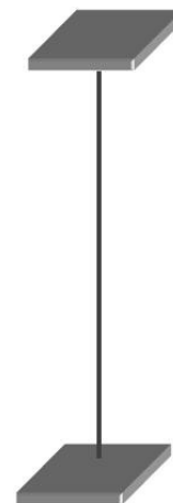
Figure 2b. Advanced ChipSat EDT concept. Each end-body has a solar panel, power supply, and an electron emitter and is capable of collecting electrons on the surface.
