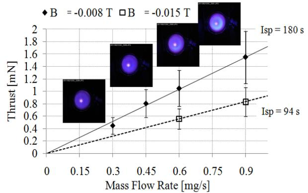
Figure 10. Correlation between a plasma emission and a thrust, changing a mass flow rate.
