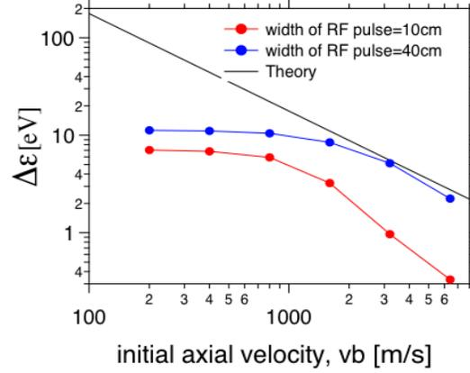
**Figure 13. Increment of ion energy  $\Delta\epsilon$  as a function of the initial axial ion velocity  $v_b$ , changing the width of RF pulse width  $L_E$  along with a theoretical line.**
