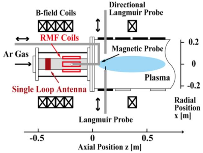
Figure 5. Experimental setup for RMF scheme in LMD.
