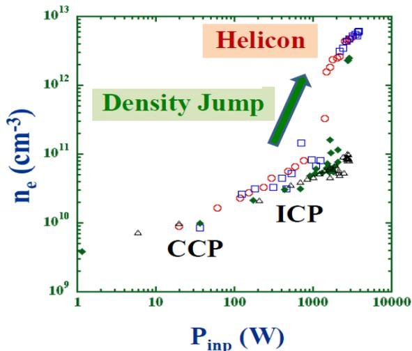
**Figure 3.** Electron density  $n_e$  as a function of the rf input power  $P_{\text{inp}}$ , changing the magnetic field near the antenna  $B_a$ .
