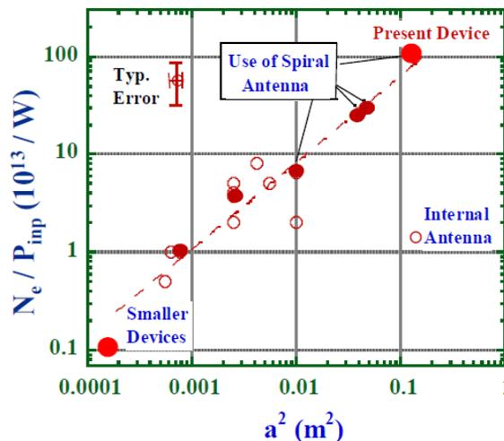
**Figure 4.**  $N_e/P_{\text{inp}}$  vs  $a^2$  for different helicon sources. Here, red closed circles show the data taken by our group.
