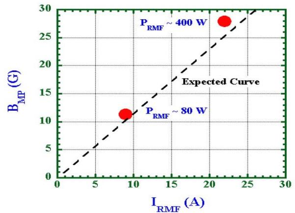
Figure 6. Magnetic probe signal  $B_{\text{MP}}$  vs. RMF current  $I_{\text{RMF}}$ .
