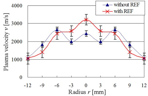
Figure 9. Ion flow velocity profile at 50 mm downstream
