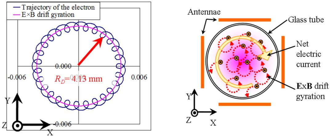
**Figure 7. (left) Trajectory of the electron under REF and uniform magnetic field:  $R_L/R_D = 0.11$  and  $\omega_{ce}/\omega = 28$ . (right) Induction of azimuthal electric current by superposition of the  $E \times B$  gyration motions.**
