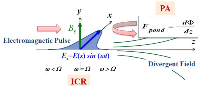
Figure 11. Concept of ICR/PA scheme.
