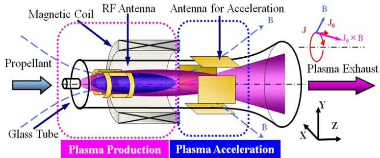
**Figure 8. Schematic of REF method using a helicon source.**
