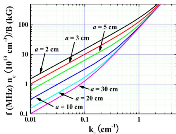
Figure 2. Dispersion relation of helicon waves.
