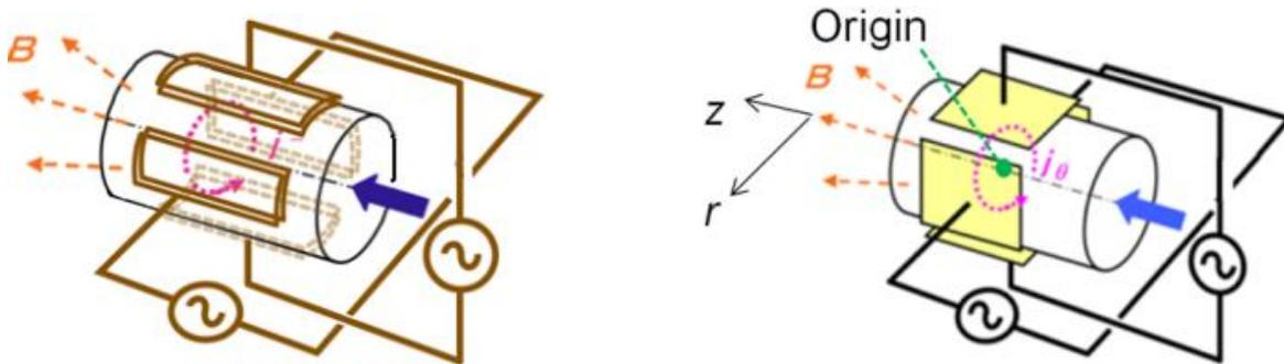
Figure 1. Configurations of (left) the RMF and (right) REF acceleration schemes.
