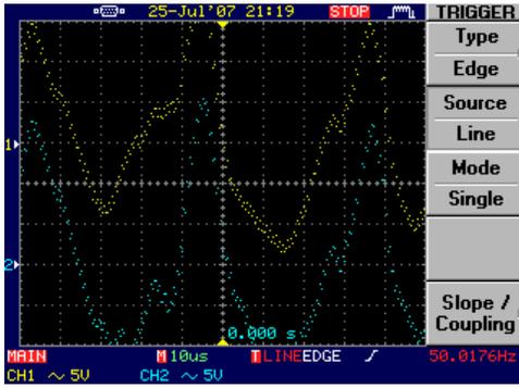
Figure 3. Oscillograms of oscillations of the plasma potential at exit of channel.
