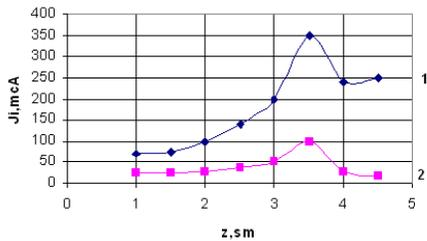
Figure 6. The dependence of direct and amplitude of alternating components of the ion current along the channel. 1-  $J_i(z)$ , 2-  $\hat{J}_i$
