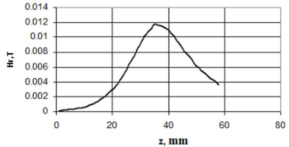
**Figure 1b. The radial component magnetic field in channel SPT.**
