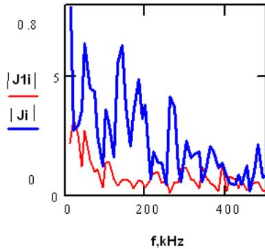
Figure 7c. The spectral composition of the low-frequency harmonic of the ion current  $J1i - z = 3.2sm, Ji - z = 3.7sm$
