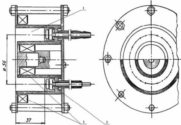
**Figure 1a. The scheme of plasma thruster SPT-70**
