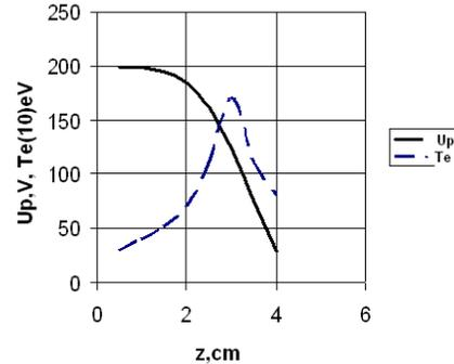
**Figure 13.** Distribution of the electrical field and electron temperature along the channel
