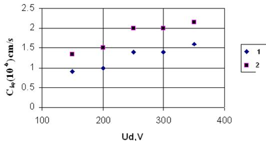
Figure.8b. Dependence of the azimuthal velocity wave  $c_{i\phi}$  on on discharge voltage (1- $z = 3.5cm$ , 2-  $z=1.2cm$ )
