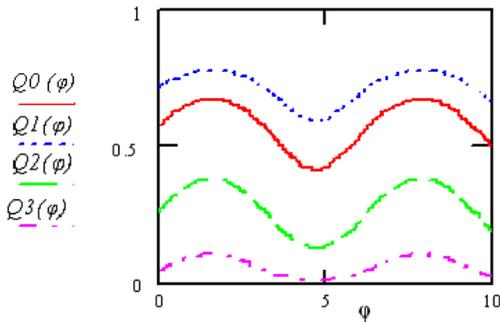
**Figure10. Change the ionization rate due to electron temperature oscillation for different values  $T_{e0}$**
