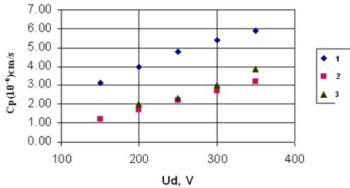
Figure 5. The dependence of the component of the phase velocity on the discharge voltage (1-longitudinal wave, 2,3-azimuthal wave)
