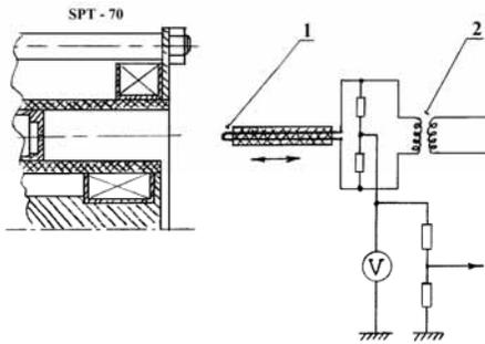
**Figure 2. Scheme for measuring the plasma potential, using a hot probe.**
