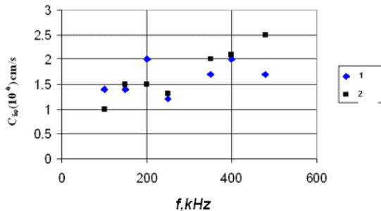
Figure 8a. Dependence of the azimuthal velocity wave  $c_{i\phi}$  on harmonic frequency  $f$  (1- $z = 3.5cm$ , 2-  $z=1.2cm$ )
