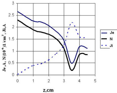
**Figure 12.** Distribution of the electron current  $J_e$ , the density of neutrals  $N$ , the ion current  $J_i$  along the channel.
