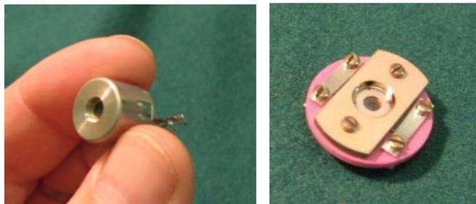
Figure 2. NCG field emission cathode (left photo) and electrode system assembly (right photo).
