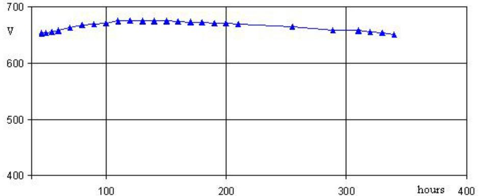
Figure 3. Field emission stability test at current stabilized at 1.4 mA.
