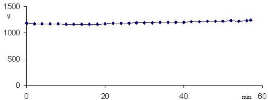
Figure 4. Field emission stability test in air at pressure of 10<sup>-4</sup> Torr.
