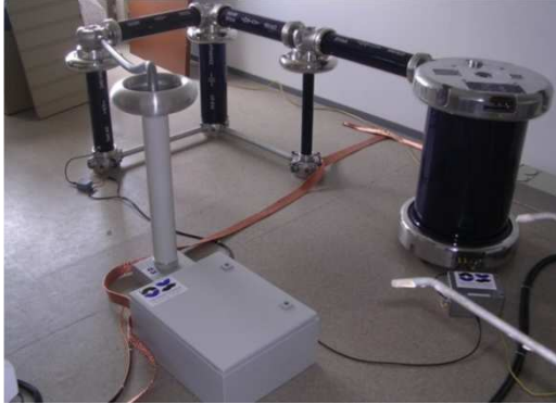
High Voltage AC/DC generator
