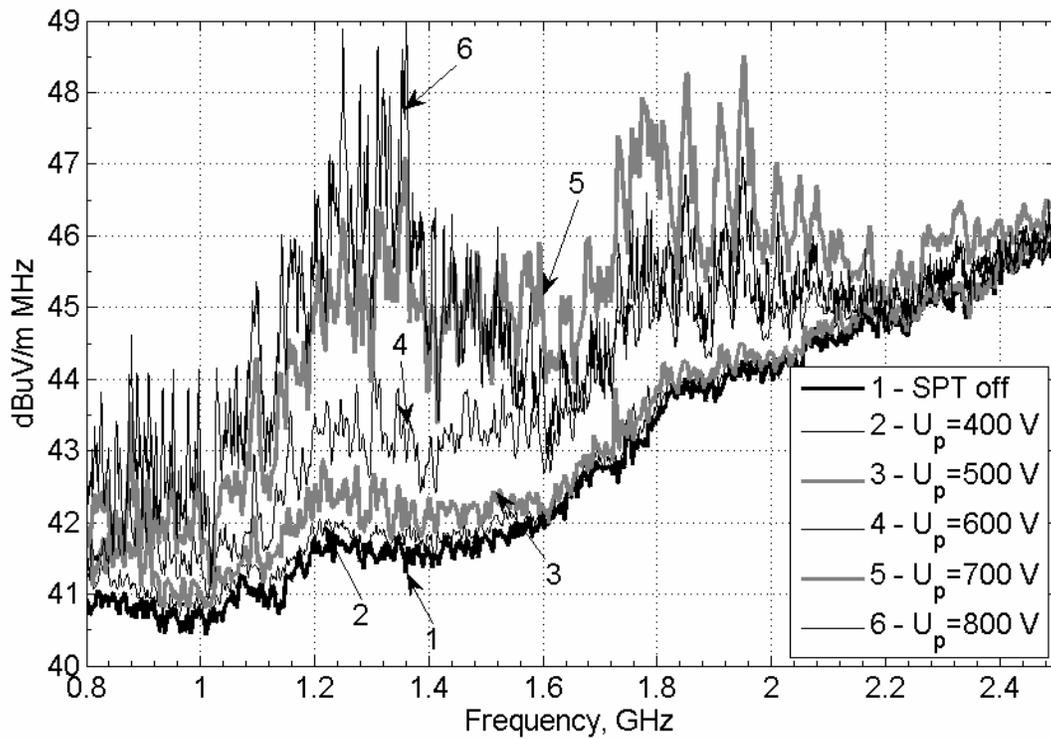
Figure 7. Discharge voltage influence on the spectral characteristics of SPT-140-1 at the mass flow rate of 5.55 mg/s.
