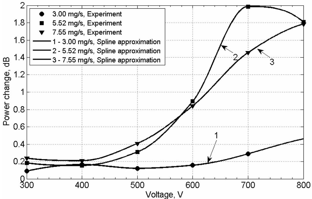
Figure 8. Relative variation of the SPT-140-1 emission power as a function of discharge voltage.
