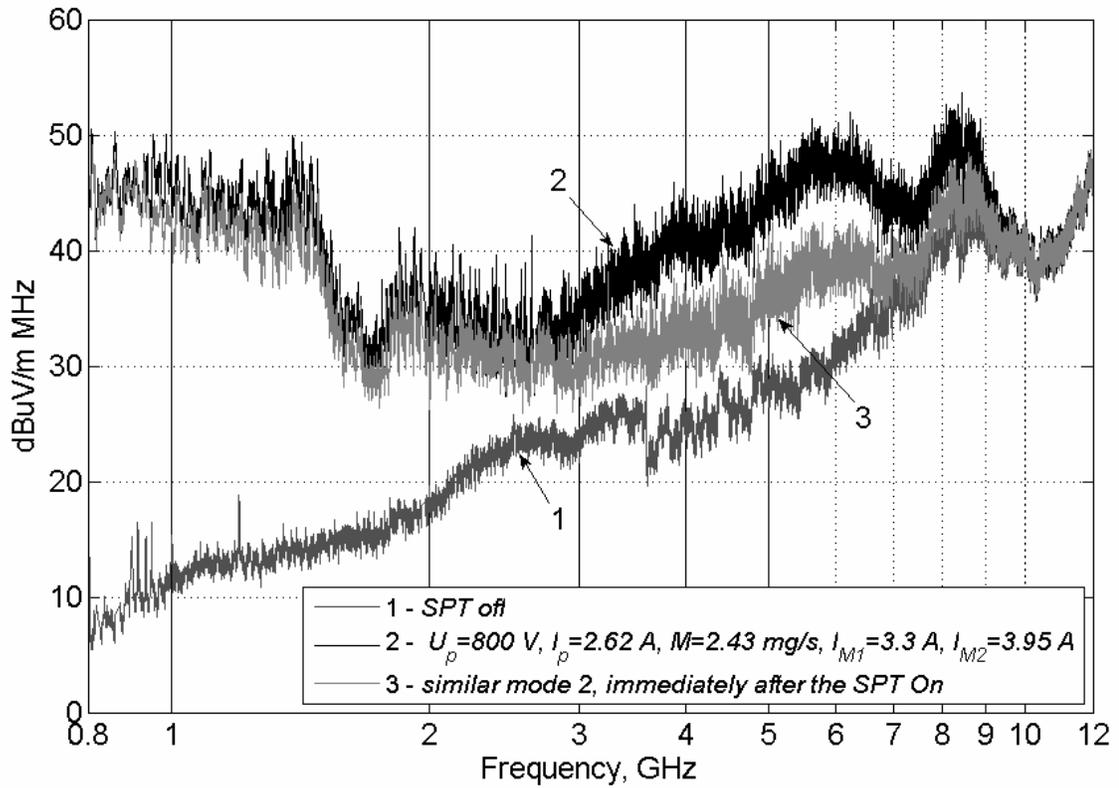
Figure 4. Variation of spectral characteristics of SPT-100-2 emission at the thruster start.
