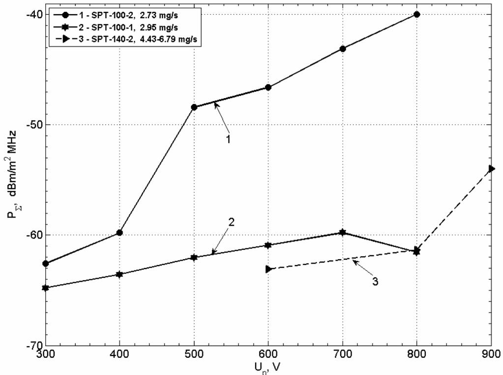
Figure 10. Power flow density at the measuring antenna input as a function of discharge voltage for different SPT models
