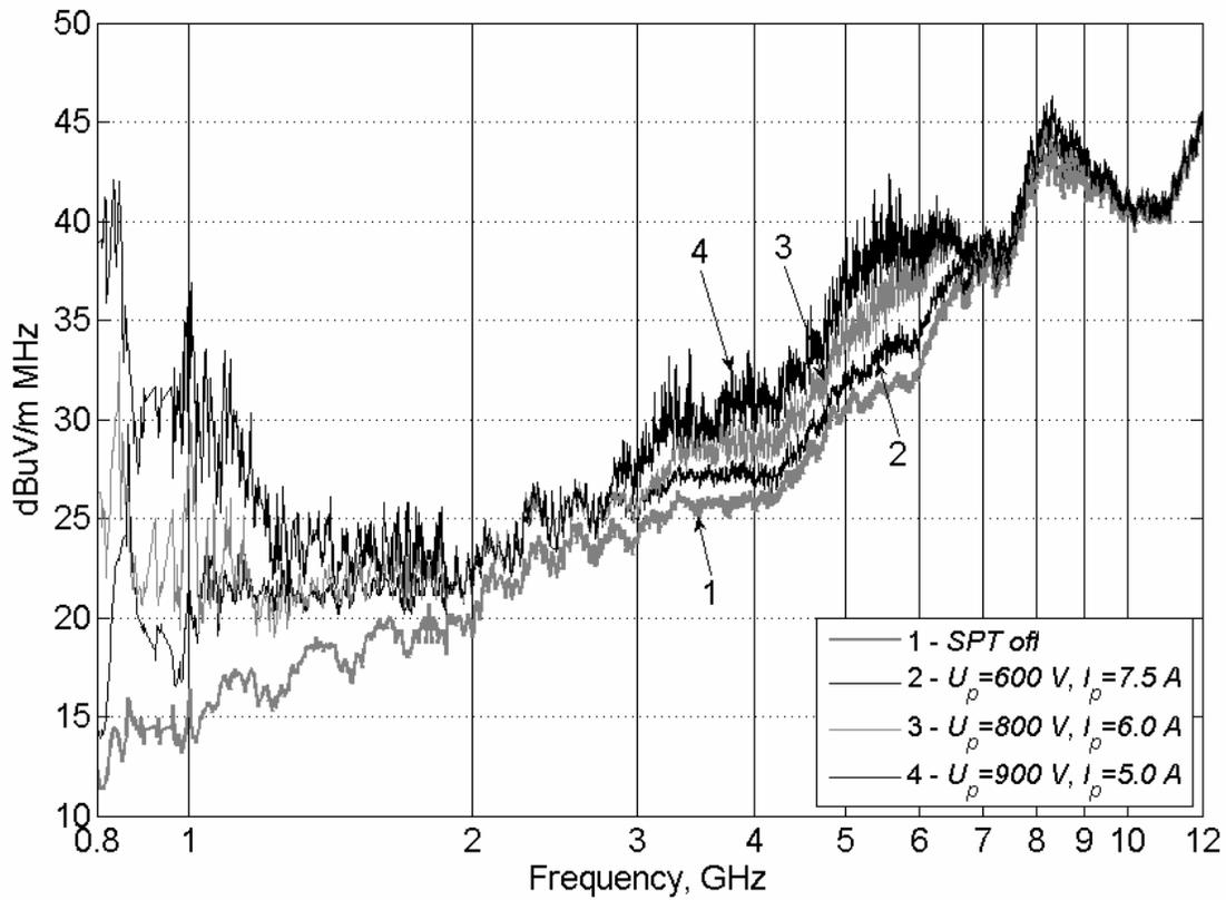
Figure 9. Spectral characteristics of SPT-140-2 emission for different discharge voltages.
