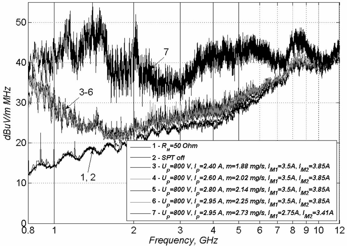
Figure 5. Influence of operation mode on the spectral characteristics of SPT-100-2 emission.
