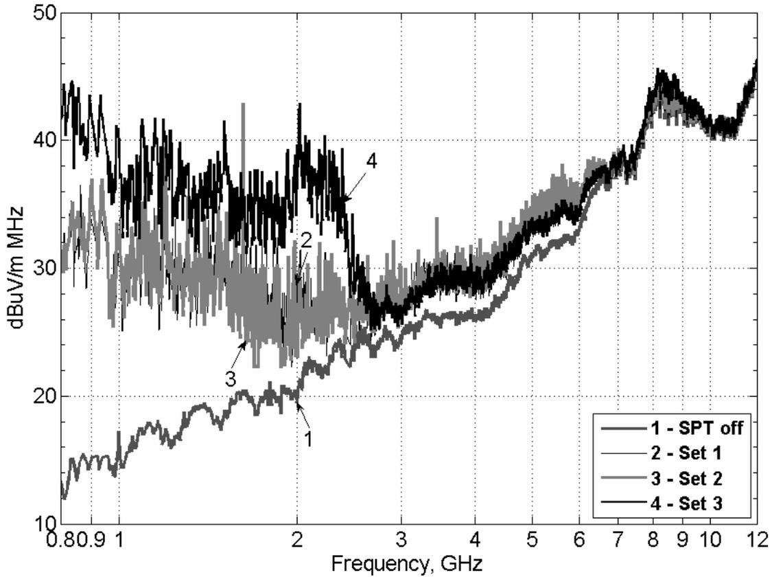
**Figure 6. Operation duration influence upon the spectral characteristics of the SPT-100-3 laboratory model emission.**
