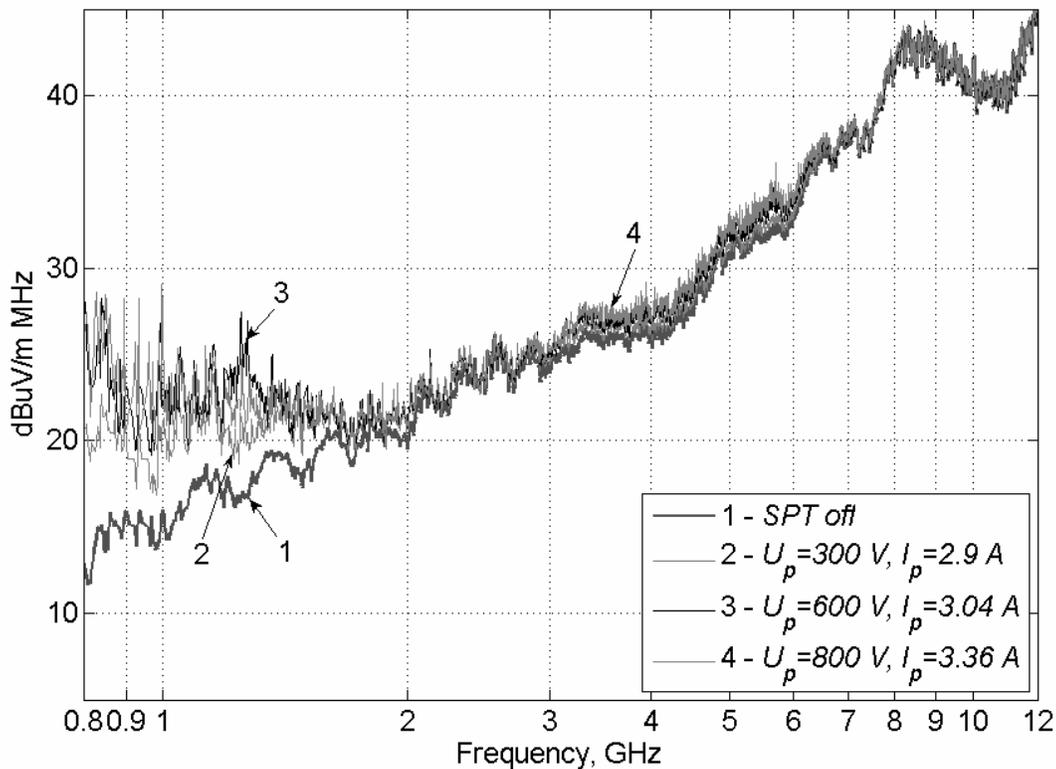
Figure 1. SPT-100-1 emission spectrum.
