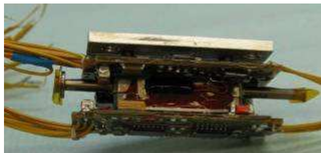
Figure 5b. MFS assembly (without external housing) showing the sandwich structure in which the MFS Fluidic sub-ass.y is placed in between the 2 small PCB's hosting the FEE
