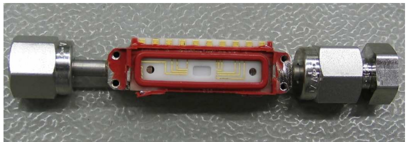
Figure 4b. Sealing O-ring placed on the \text{Al}_2\text{O}_3 support
