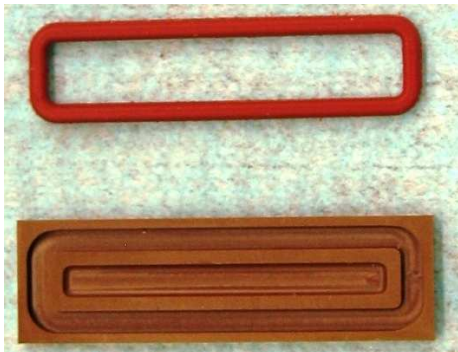
Figure 4a. Pre-built o-ring (upper image) to be accommodated in the vespel gas duct (lower image)
