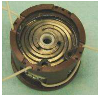
Figure 1b. Piezo ceramic actuator based on a set of piezo ring piezo-ceramic benders
