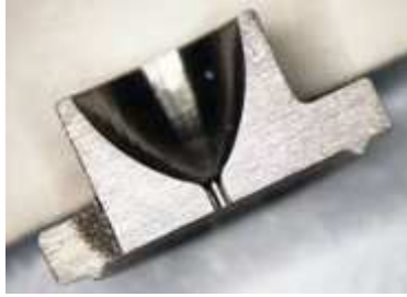
Figure 2a. LP TV Nozzle (cutaway) close up
