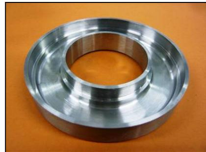
**Figure II-1: up-stream part of a discharge chamber**
