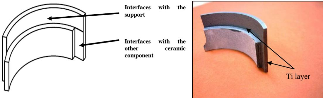
**Figure II-2: Ceramic single component of the DC ring**
