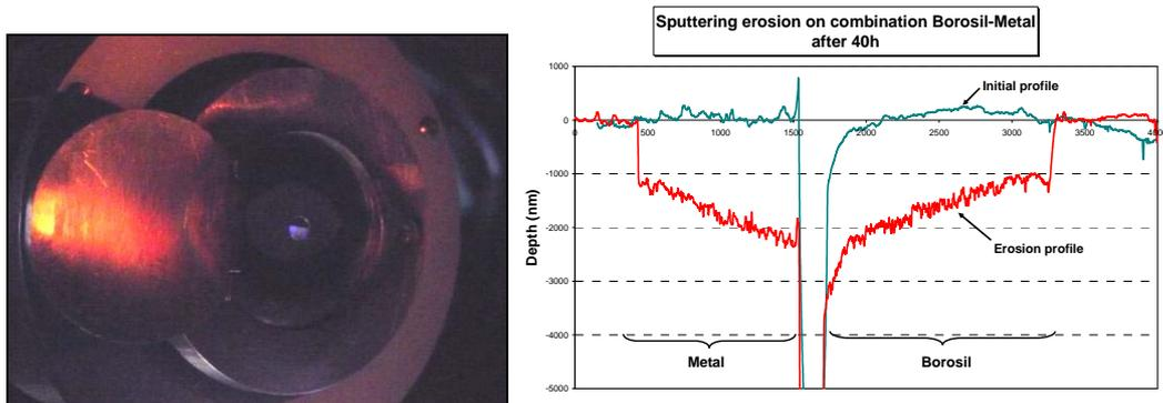
**Figure II-6: Erosion profile of metal-ceramic interface**
