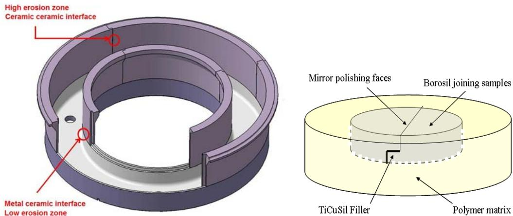
**Figure II-5: erosion zones and test sample**
