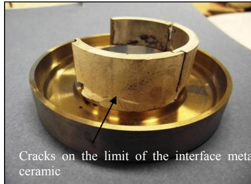
**Figure II-3: failure on the technical demonstrator**
