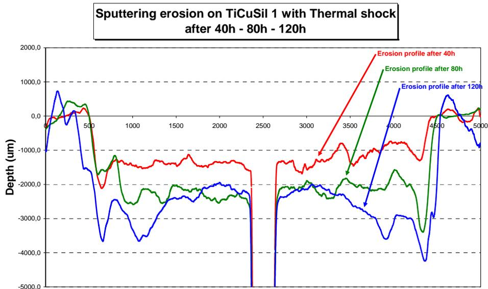
**Figure II-8: Erosion profile of ceramic-ceramic interface**
