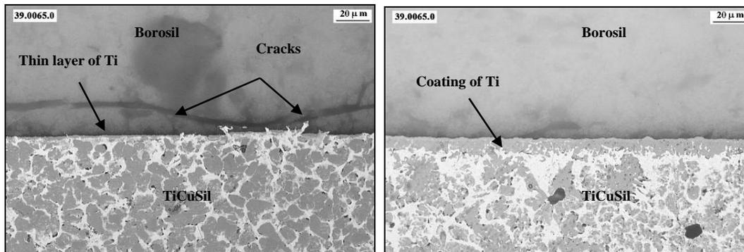
**Figure II-4: Ceramic joining without and with accommodation layer of Ti**
