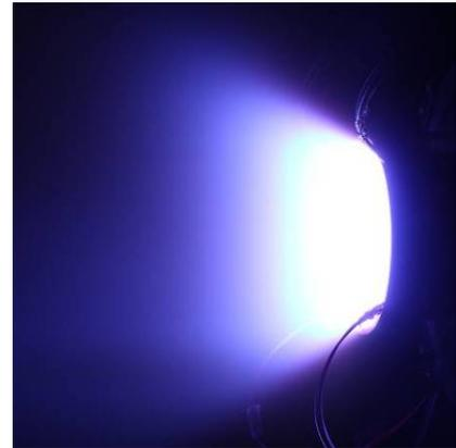
**Figure 1: MPD thruster firing**
