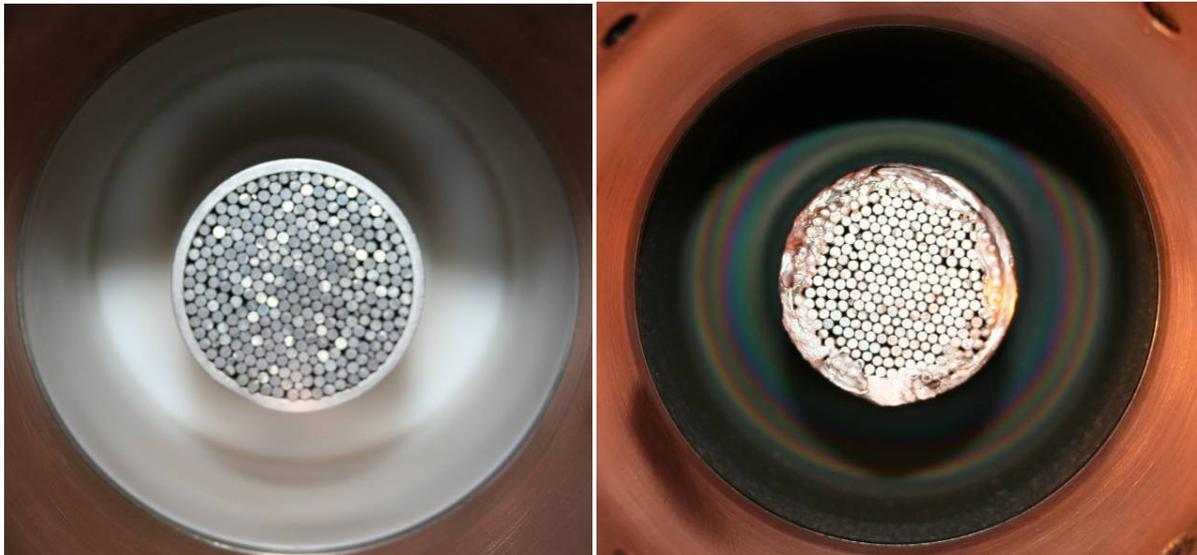
Figure 14: McHc at the beginning of life (left) and after about 200 shots (right)
