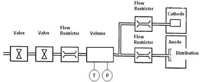
**Figure 3. Fluid management sketch.** *The fluid management device dispatch with only three restrictors, two on-off valves, one pressure transducer, one temperature probe, volumes and tubing the gas from the main tank to the thruster.*
