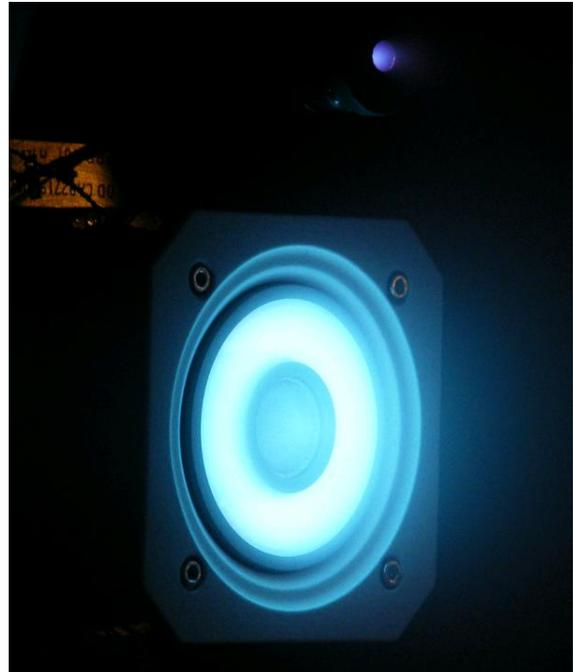
**Figure 5. PPS@X00 prototype N°1 firing.** Firing performed on the LIB Snecma test bench.
