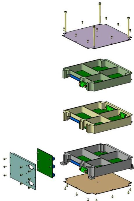
**Figure 4. Power Processing Unit.** *View of the inside of the PPU able of 500W management.*
