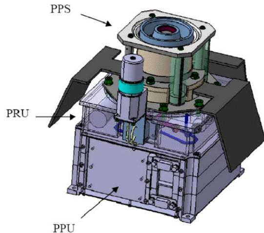
**Figure 1. Compact Hall Effect Assembly Propulsion subsystem.** Overall dimensions are 150x150x220 without radiation panels and cathode.
