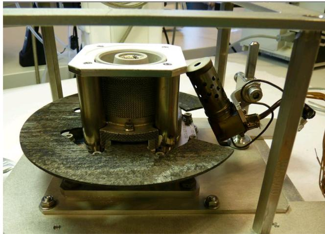
**Figure 2. PPS@X00 prototype n°1.** *The thruster is mounted in its handling tooling, we can see the radiation device (in carbon-carbon) specific to the test bench, the cathode is not in its definitive place.*
