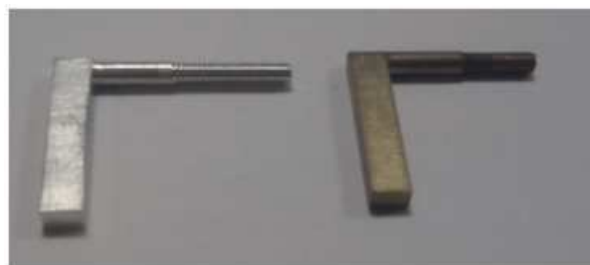
Figure 6. Contact arms. Left: Aluminium, Right: Elkonite
