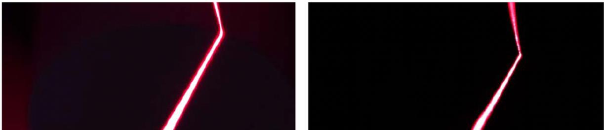
Fig. 11: Laser light projected on the inner edge of BN channel – at the beginning of life (left), after 450h (right)
