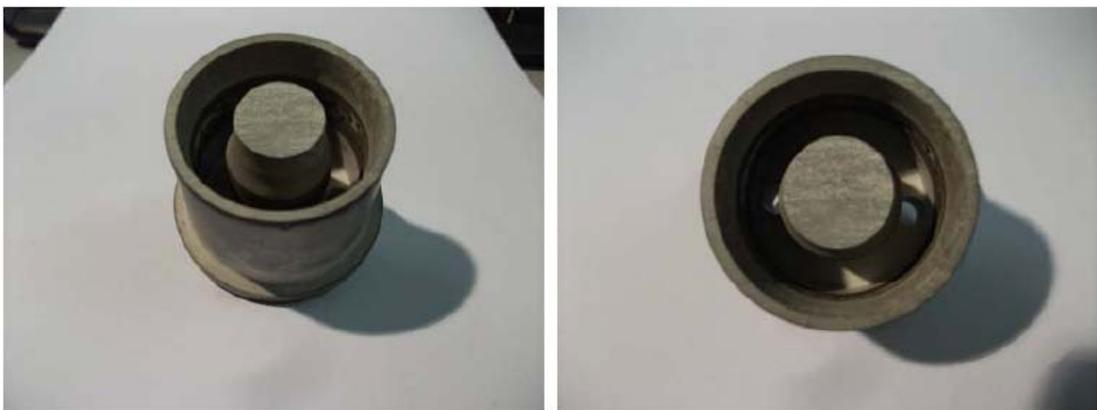
**Fig. 13: BN ceramic channel after 450 hrs of operation**
