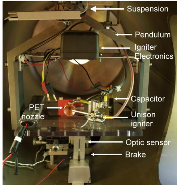
Figure 4. Experimental setup on the impulse pendulum at IRS.
