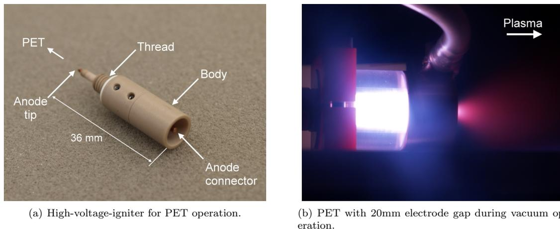
**Figure 3. HV-igniter and PET operation.**
