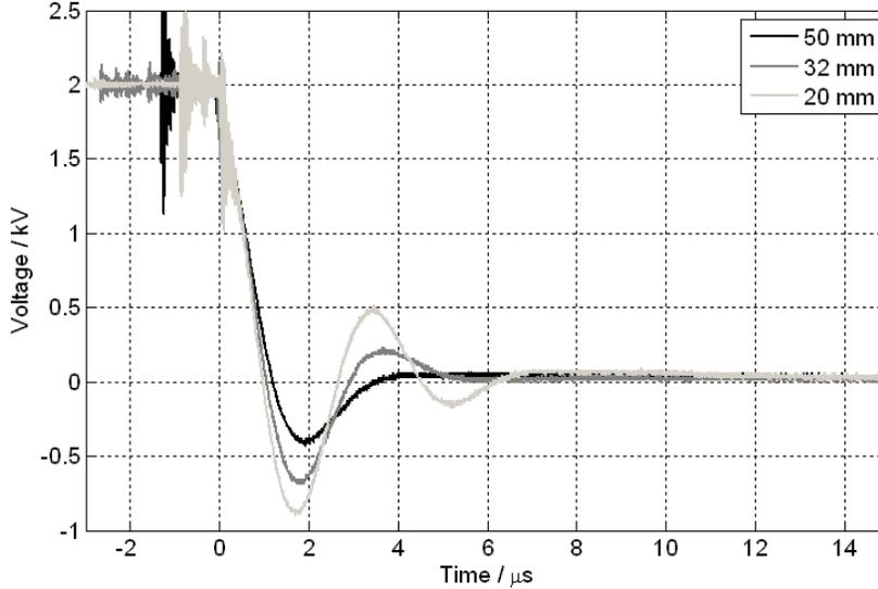
Figure 5. Influence of  $x_{gap}$ -variation on PET temporal discharge voltage for 3J pulse energy.
