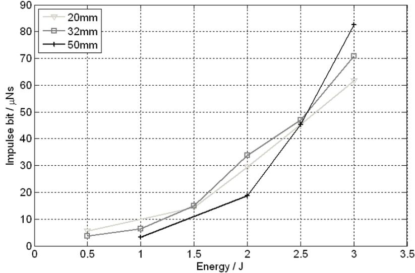
Figure 6. Impulse bit over pulse energy for variation of the electrode gap.
