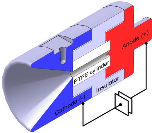
(a) Thruster setup of a PET.
