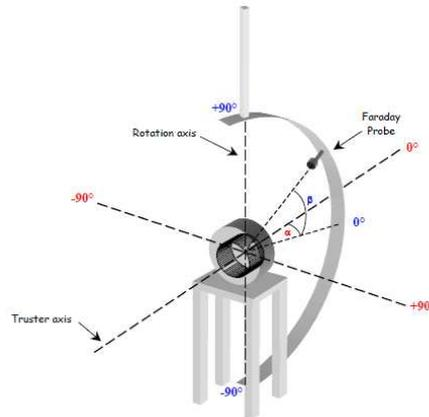
**Figure 2. Schematics of the LVTF-1 beam diagnostic system**
