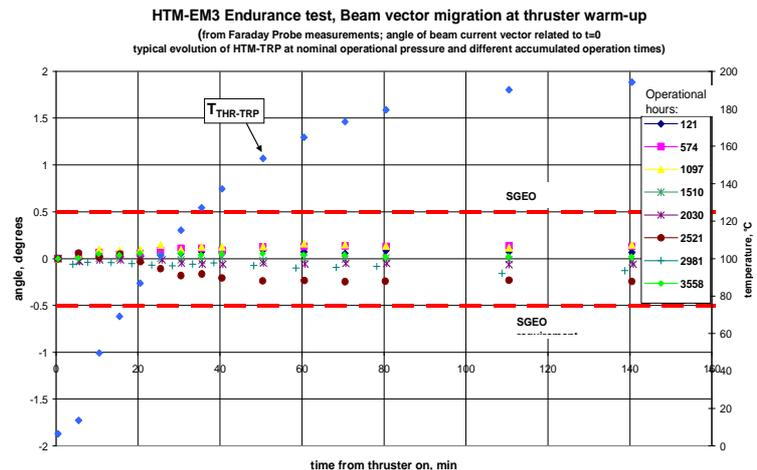
**Figure 10. Beam current vector migration during thruster warm-up at different accumulated operation times during Endurance test**
