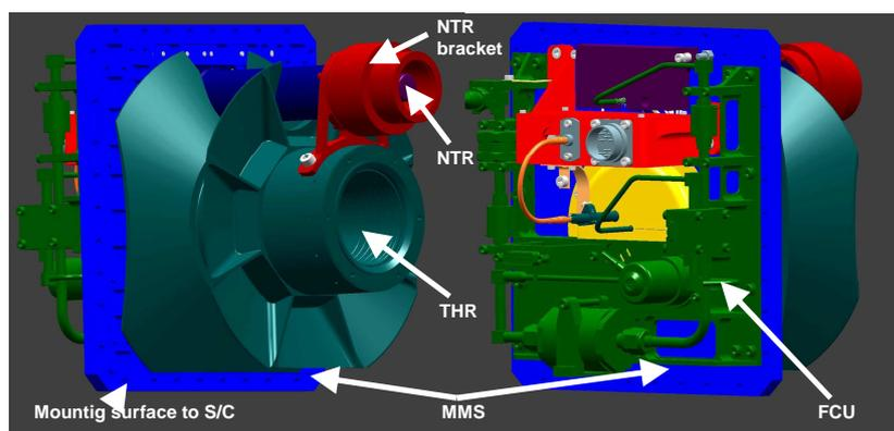
**Figure 1. 3D-drawing of the HEMPT Module. Left: front side; right: rear side.**
