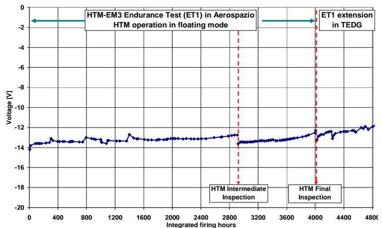
Figure 15. Keeper ignition voltage evolution with firing time in Endurance Test 1 and ET1 extension.
