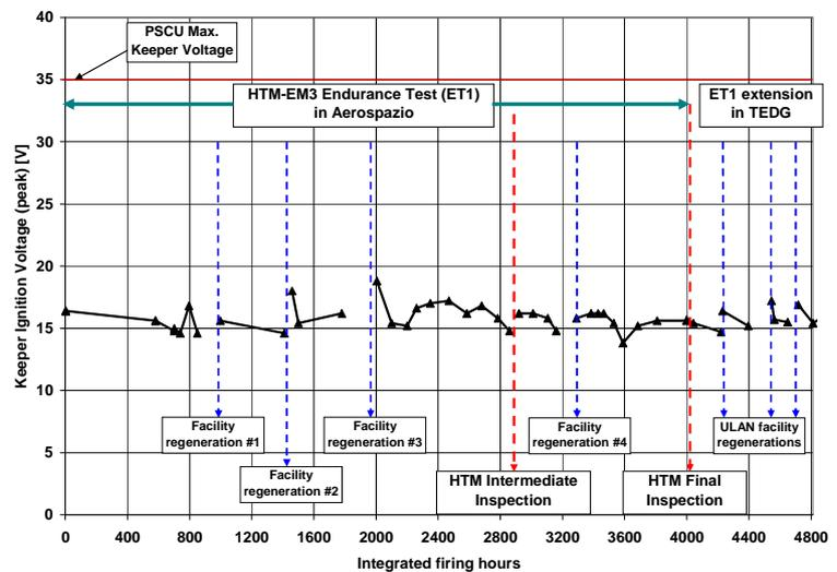
Figure 14. Cathode-to-ground coupling voltage evolution with firing time in Endurance Test 1 and ET1 extension.
