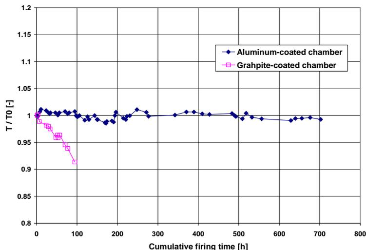
Figure 13. THR-EM5 thrust evolution with firing time as a function of chamber-wall material in the test facility ULAN at TEDG.
