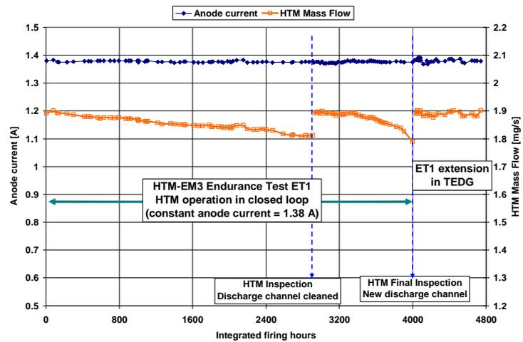
Figure 6. HTM mass flow evolution with firing time in Endurance Test 1 and ET1 extension.
