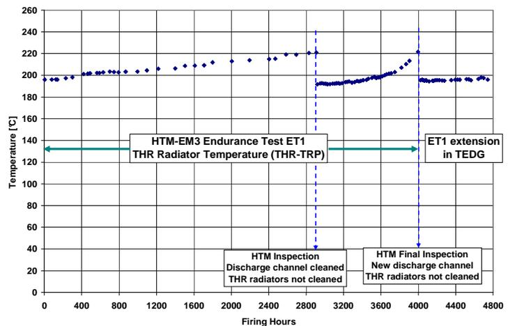
Figure 8. THR radiator temperature evolution with firing time in Endurance Test 1 and ET1 extension.
