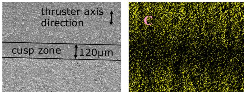
Figure 11. SEM image (left) and EDX mapping of carbon (right) in the cusp region of the thruster discharge channel after ET1.
