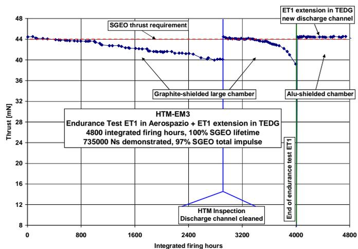
**Figure 5. Thrust evolution with firing time in Endurance Test 1 and ET1 extension.**
