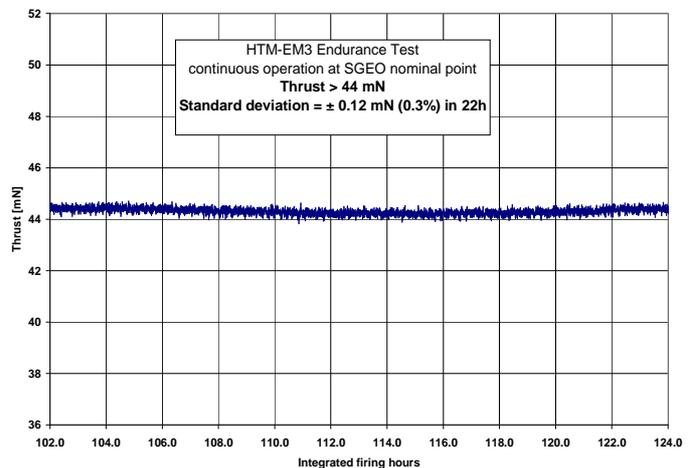
**Figure 4. HTM continuous operation @ SGEO working point.**
