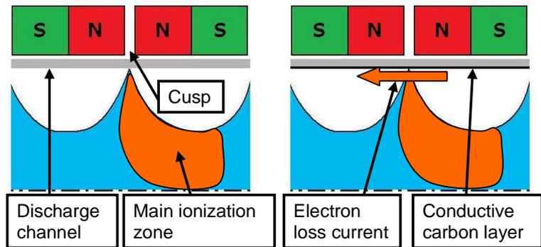
Figure 7. Schematic of thruster cusp region at BOL (left) and at the intermediate inspection (right).
