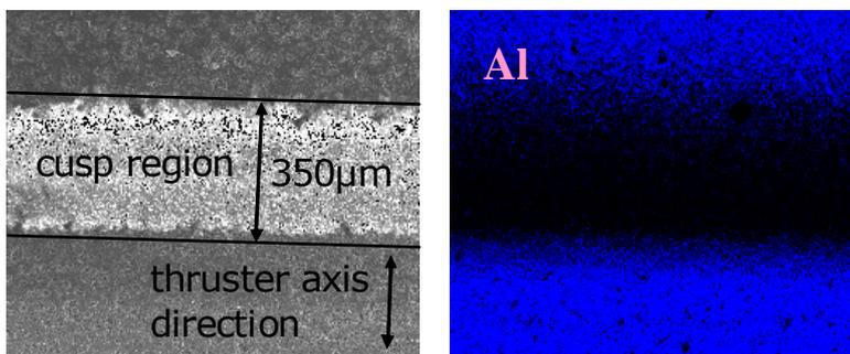
Figure 12. SEM image (left) and EDX mapping of aluminum (right) in the cusp region of the thruster discharge channel operated in the aluminum-coated ULAN test facility at TEDG
