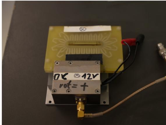
Figure 4. Example of a HOKA Current Sensor.<sup>15</sup>
