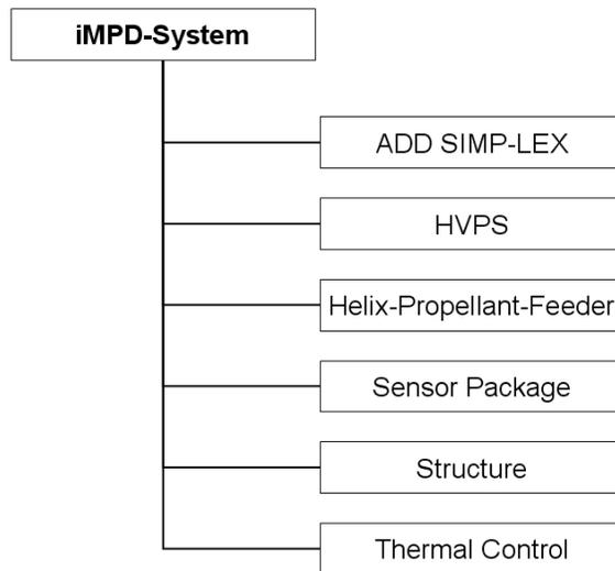
Figure 3. Component breakdown of the iMPD-system.
