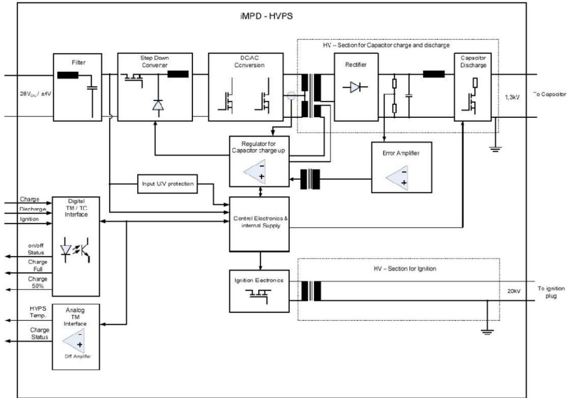
Figure 8. PPU block diagram
