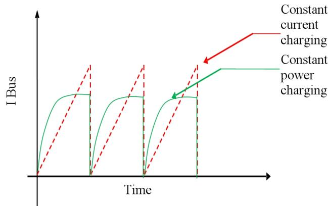
Figure 7. Input current of PPU comparing different charging methods.
