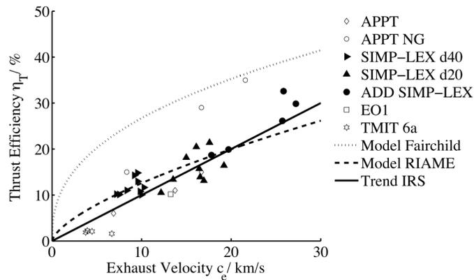
Figure 1. Thrust efficiency against exhaust velocity for different PPTs.<sup>15</sup>
