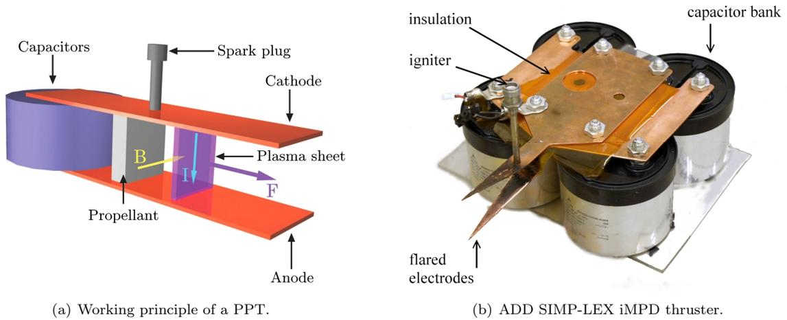
Figure 2. ADD SIMP-LEX thruster and working principle.
