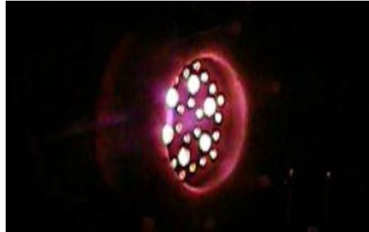
Figure 9. MMIT firing into the vacuum chamber.
