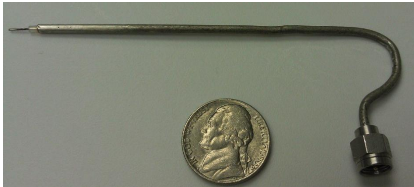
Figure 7. Langmuir probe used in testing the MMIT.
