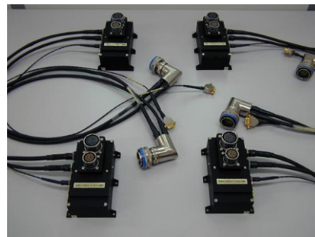
Figure 11. Electrical Filtering Units (right and left configurations).
