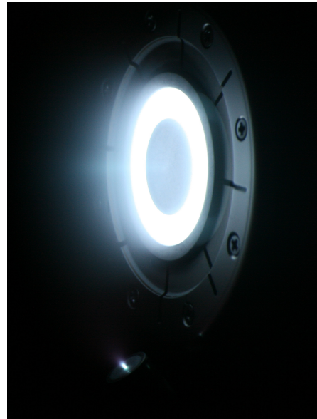
Figure 11. The HT-100b with KhAI cathode during test
