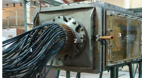
Figure 2. Experimental facility. 1-cable bridge, 2- vacuum feeder, 3 - vacuum chamber.
