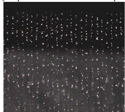
Figure 6. A Cloud of molybdenum micropowder. The average size of particles, 70 microns.
