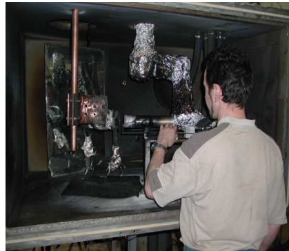
Figure 3. 2000A cathode installed in vacuum chamber a) and its working b).
