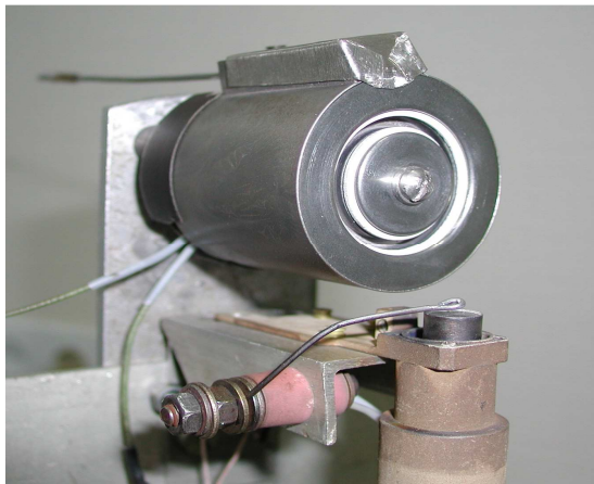
Figure 1. General view of laboratory model of low-power Thruster with Anode Layer TAL-23.
