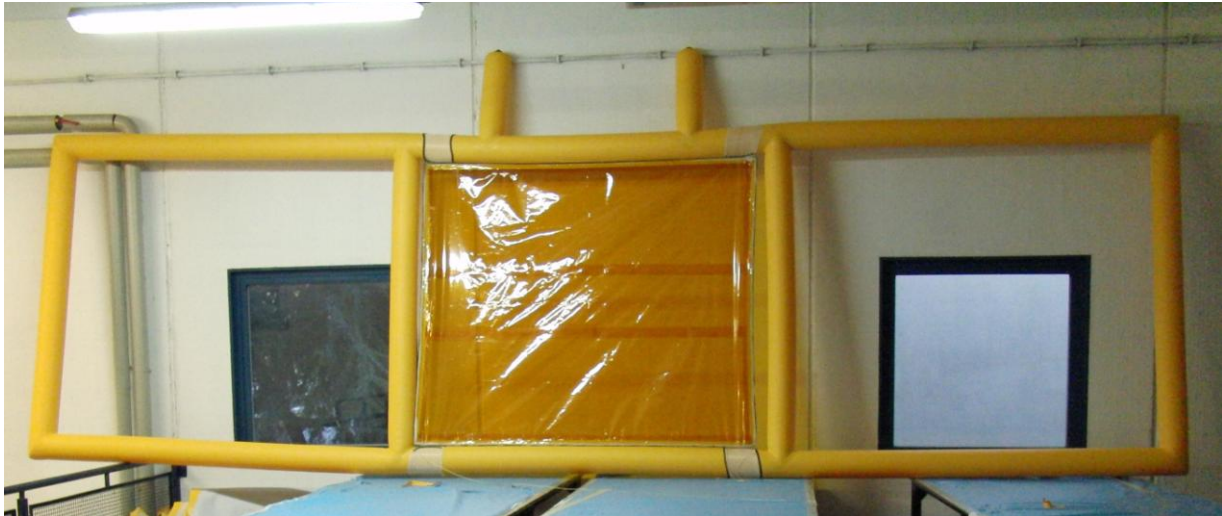
Figure 5. Solar Generator Breadboard Model composed of only 3 elements
