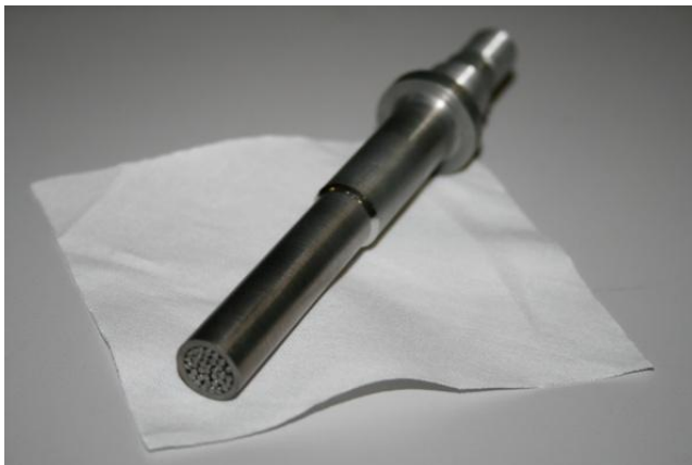
Figure 11. Alta multichannel 180 A cathode (on the left) and during the test campaign @ Alta
