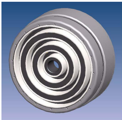
(a) Design of the 11 kW Multi-channel Hall Thruster Mc-HT (Alta)
