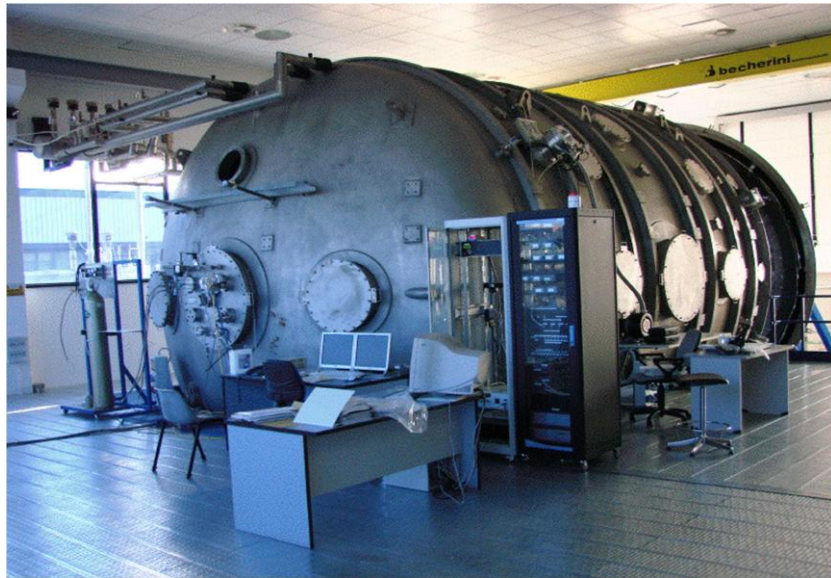
Figure 14. Alta IV10 Space Simulator
