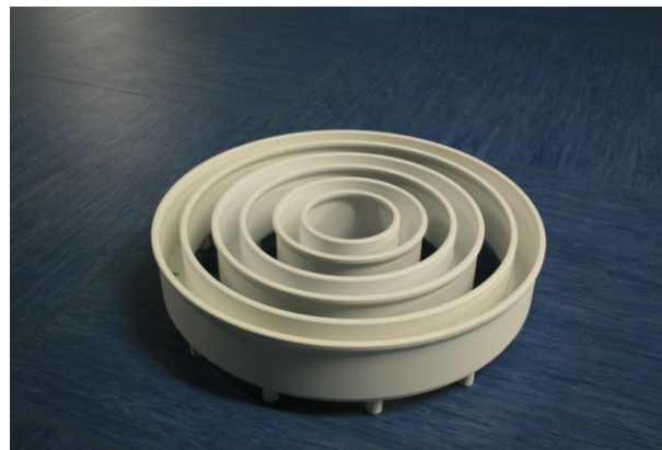
(b) Anode discharge chambers for the 11 kW Mc-HT (Alta)
