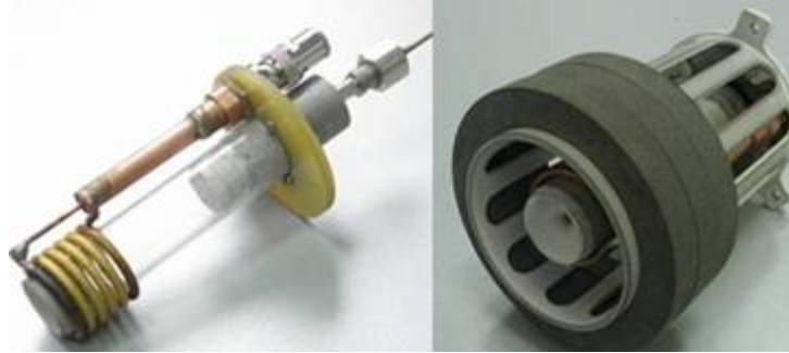
Figure 41. Photos of EM 01 without case (left) and EM 02 with case and permanent magnets set (right)
