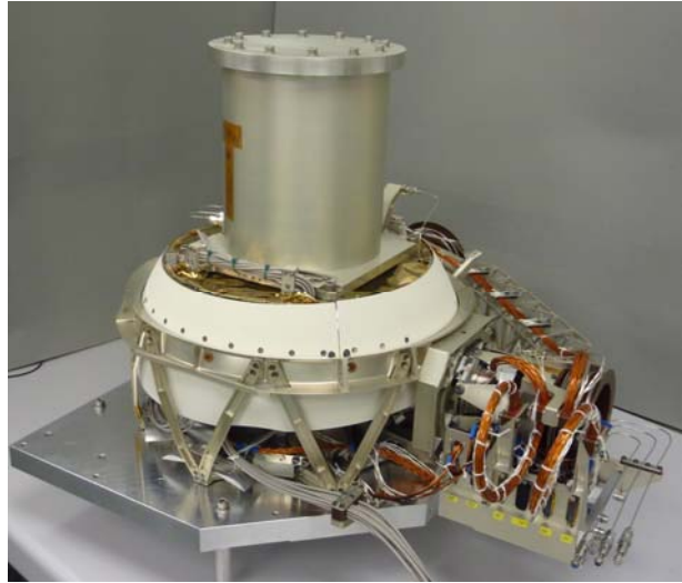
Figure 7. Thruster Pointing Mechanism (TPM) with Thruster Mass Dummy and Sun-Shield attached.
