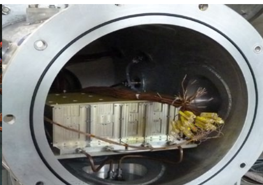
Figure 11: Photograph of the CPE brassboard PPU inside VF70.
