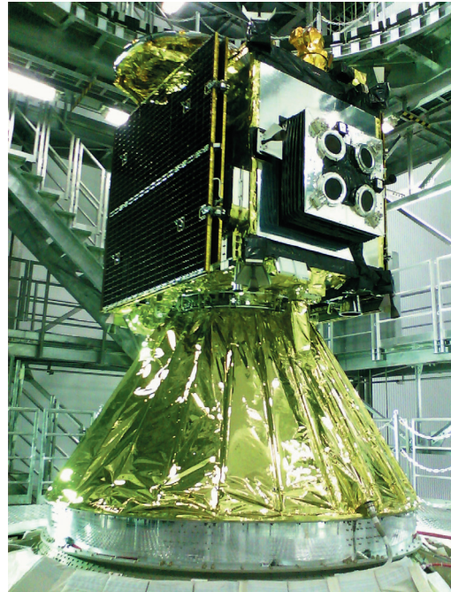
Figure 4. Four microwave discharge ion engines onboard Hayabusa2 asteroid explorer on PAF of H2A rocket.
