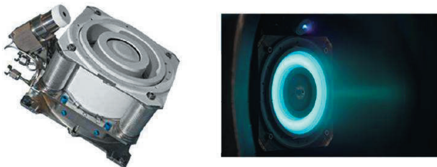
Figure 3. PPS®1350-E thruster on stage and during ground qualification test. Credits : SNECMA
