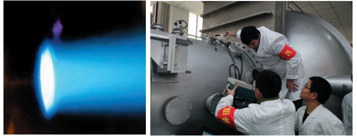
Fig. 3 Thruster Working and Resistance Measurement
