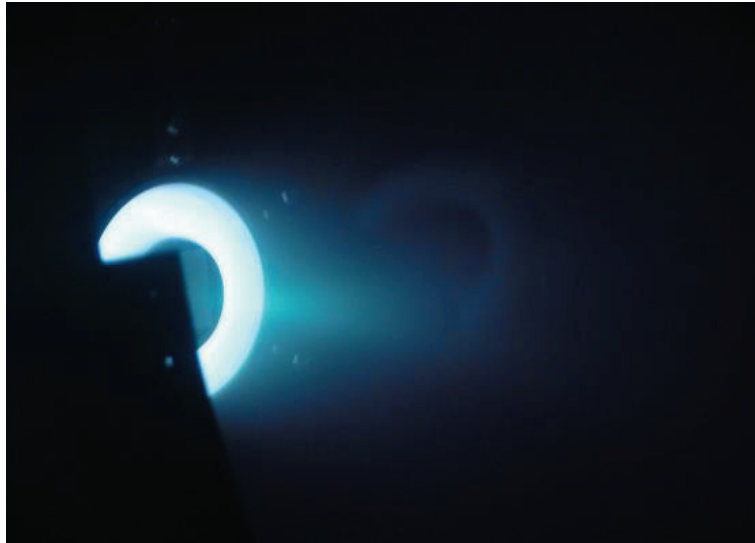
Figure 12. Operation photo at discharge voltage of 300 V.
