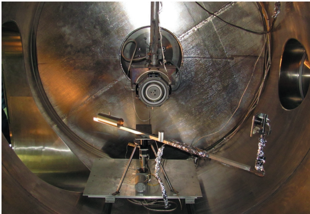
Figure 4. PlaS-120CM ser.01 in vacuum chamber of the Y-2B-2 test facility with the probe movement device
