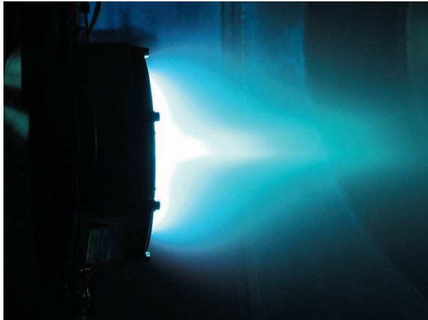
Figure 6. PlaS-120CM plasma plume during operating at operating point with U_d=300 V and I_d=18.3 A
