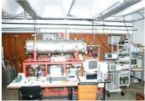
Figure 1. General experimental setup with vacuum chamber and diagnostics for Hall thruster tests.
