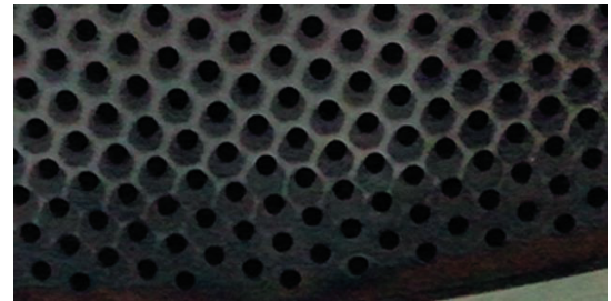
Figure 14. The edge of accelerating grid of the ion thruster IT-500.
