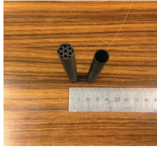
Figure 13. Hollow cathodes (Left: multi hollow cathode; Right: single hollow cathode).
