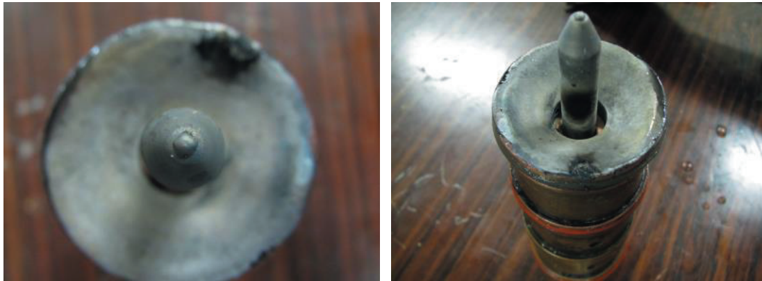
Figure 10. The damage in cathode tip.
