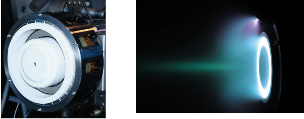
Figure 3: The HT5k thruster mounted on the thrust balance (left) and during operation (right).
