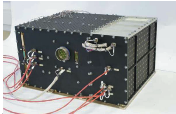
Fig. 7 GOCE IPCU - Mass: 17 kg – Size: 380 x 270 x 205 mm 3
