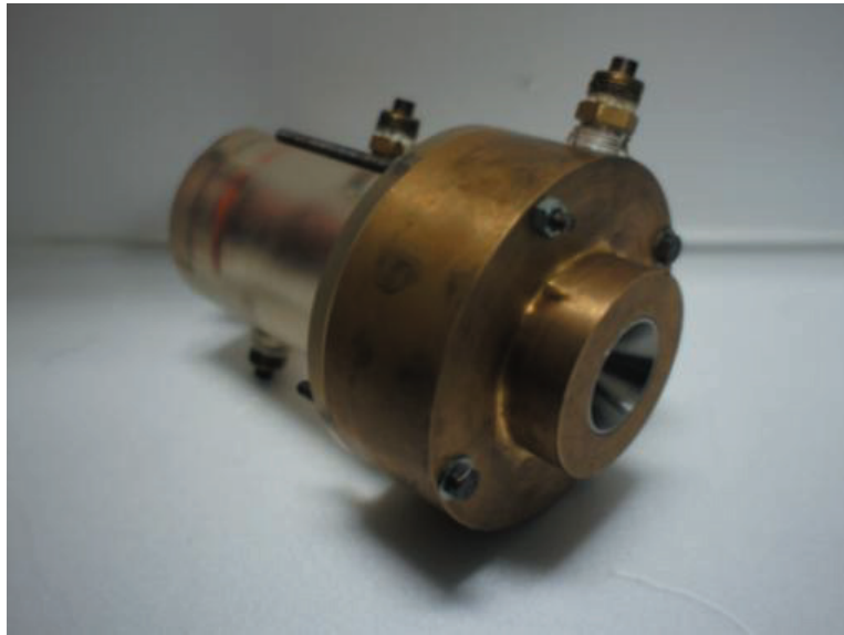
Figure 3. Photo of low-power arcjet thruster.
