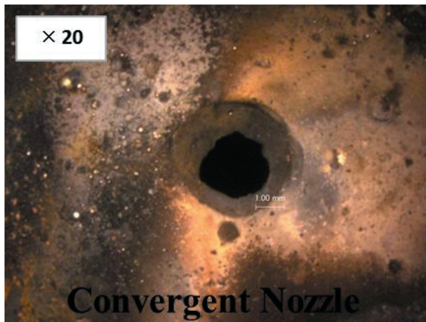
Figure 22. Photo of anode convergent nozzle after experiments.
