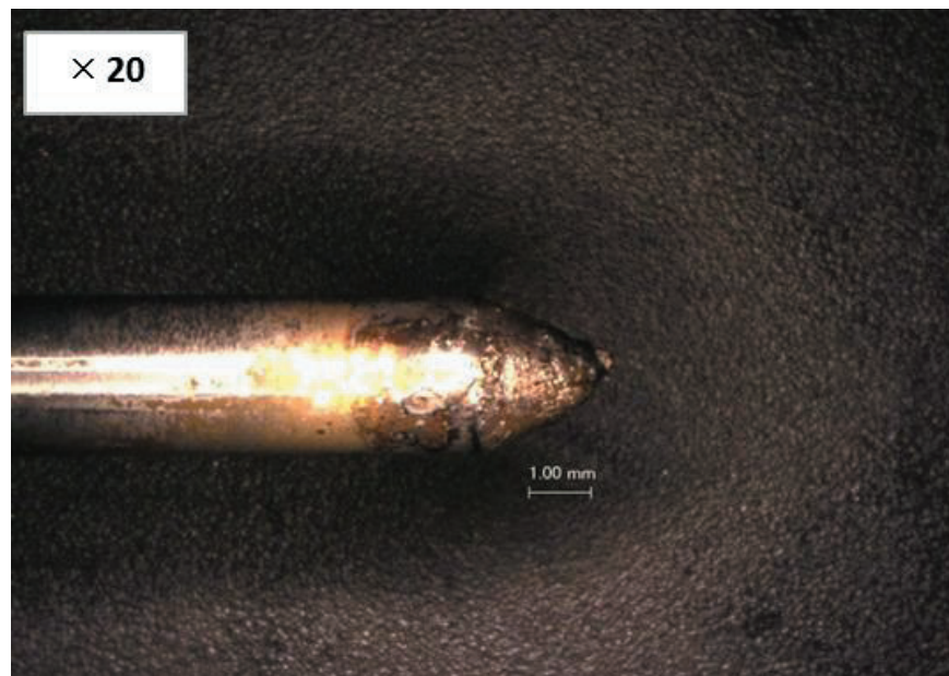
Figure 24. Photo of cathode after experiments.
